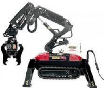
Figure 9 a) Remote Control Excavator
