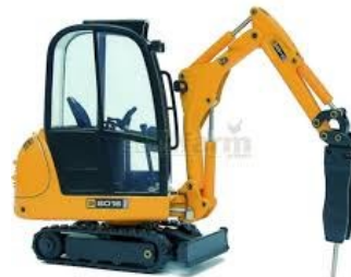
b) Excavator with Pneumatic Hammer
