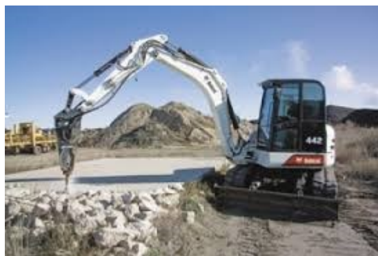
b) Small Excavator for Demolition
