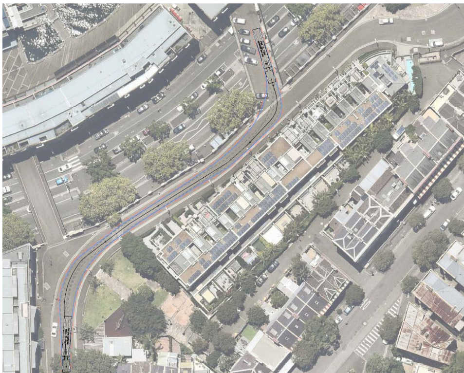
Figure 2: Swept path, 19-metre semi-articulated vehicle exit
