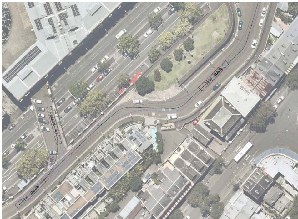
Figure 2: Swept path, 19-metre semi-articulated vehicle exit
