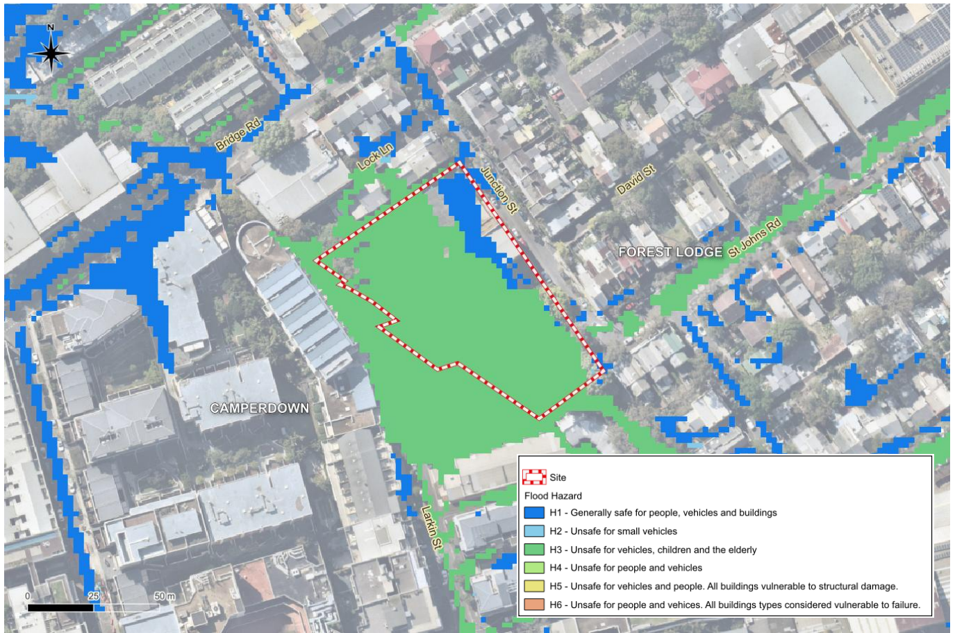
Figure 3-3: Existing Flood Hazard 1% AEP Flood Event
