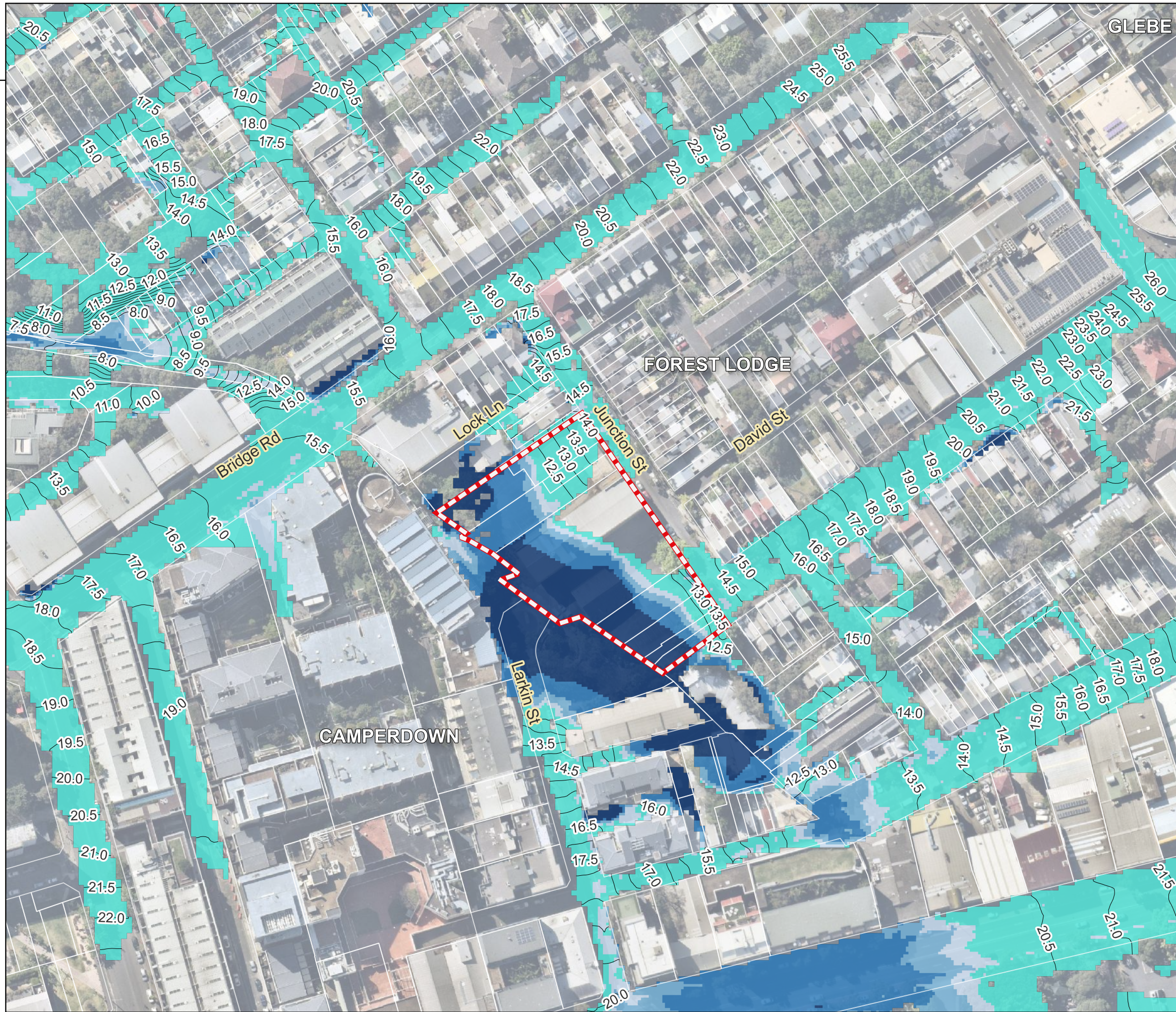
2-32 Junction Street Flood Impact Assessment Figure 01 20% AEP Existing Peak Depth and Water Level Contours
