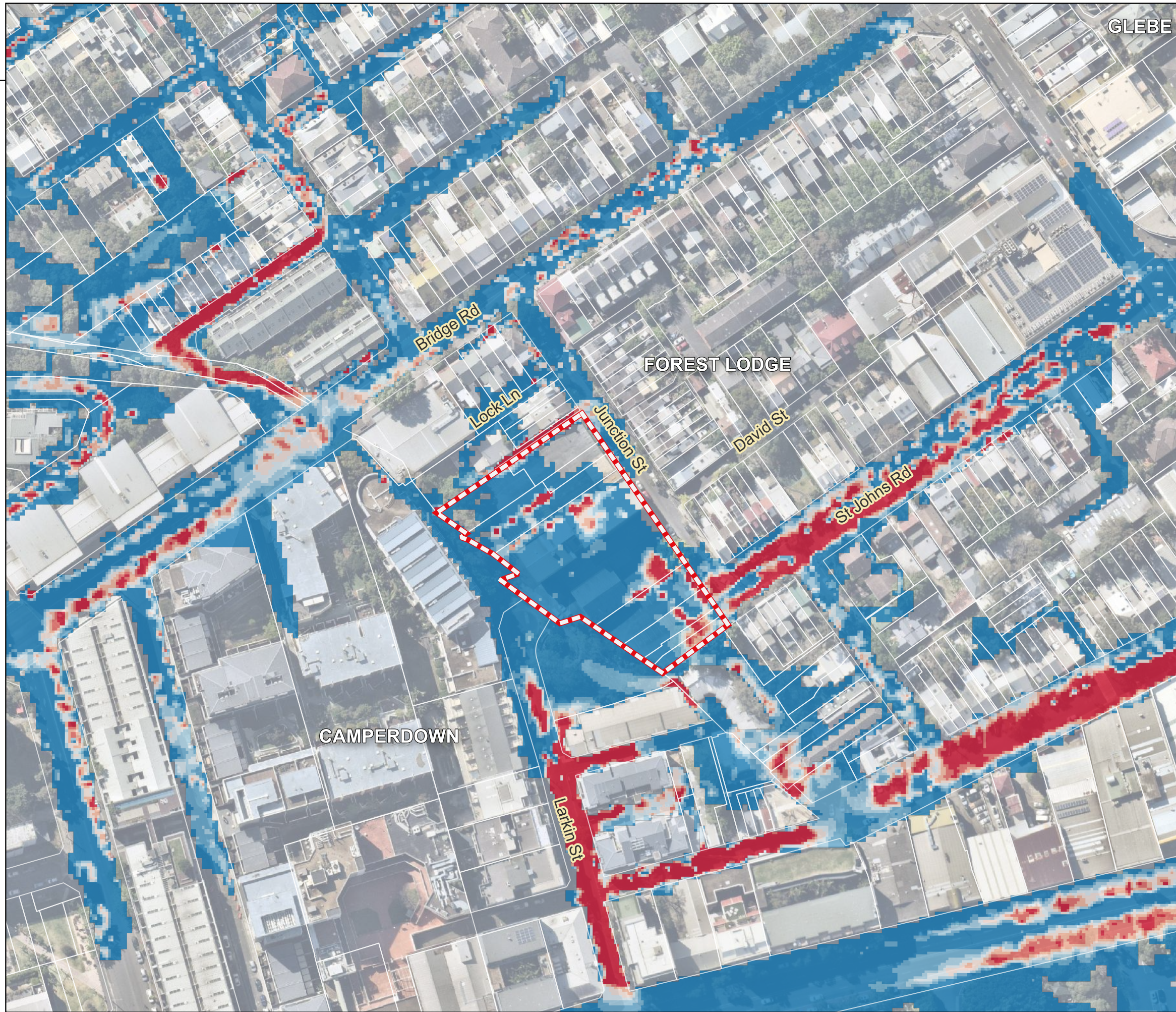
2-32 Junction Street Flood Impact Assessment Figure 41 1% AEP Post-Development Peak Velocity
