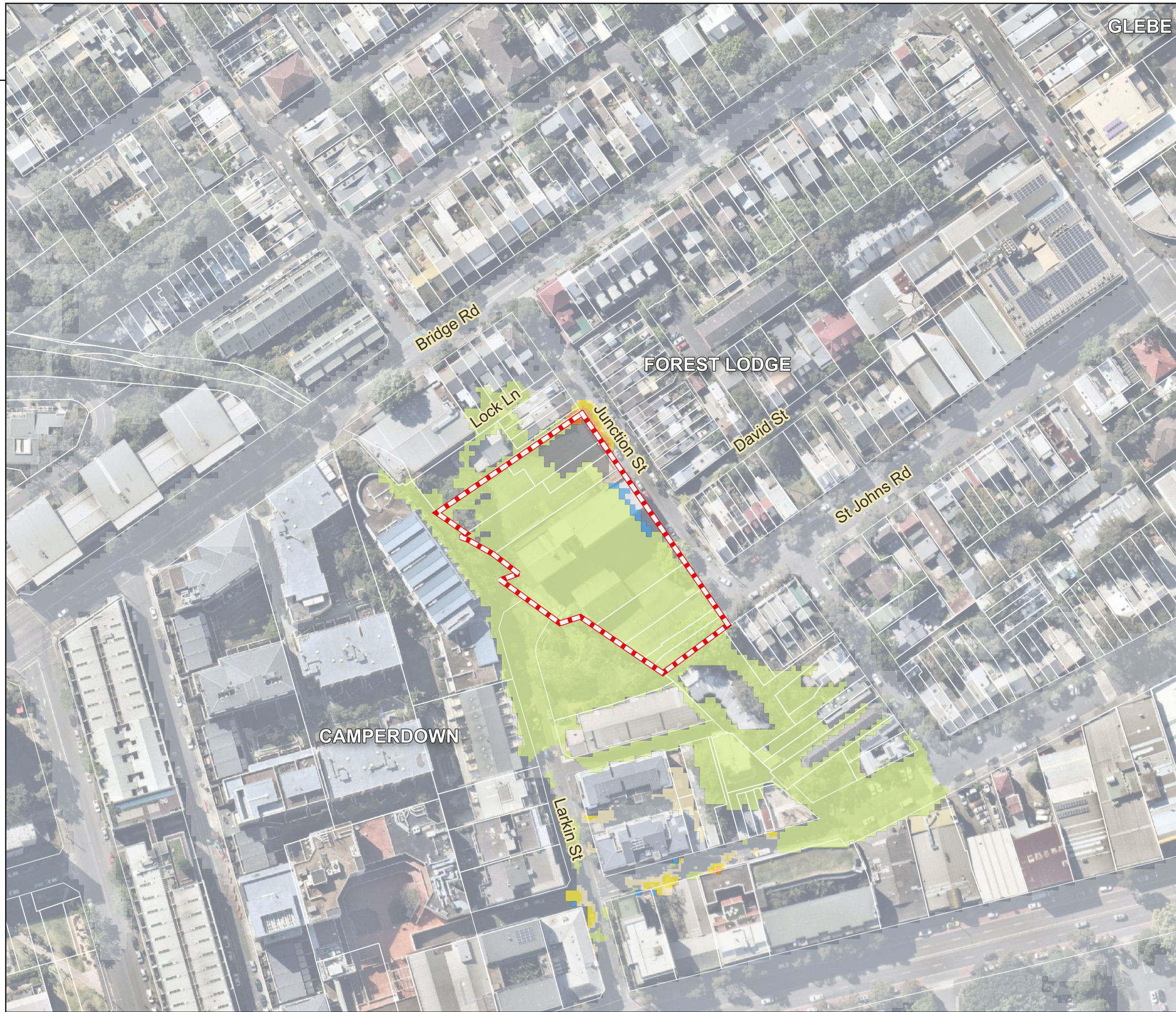
2-32 Junction Street Flood Impact Assessment Figure 59 1% AEP Change in Water Level (Post-Development less Existing)
