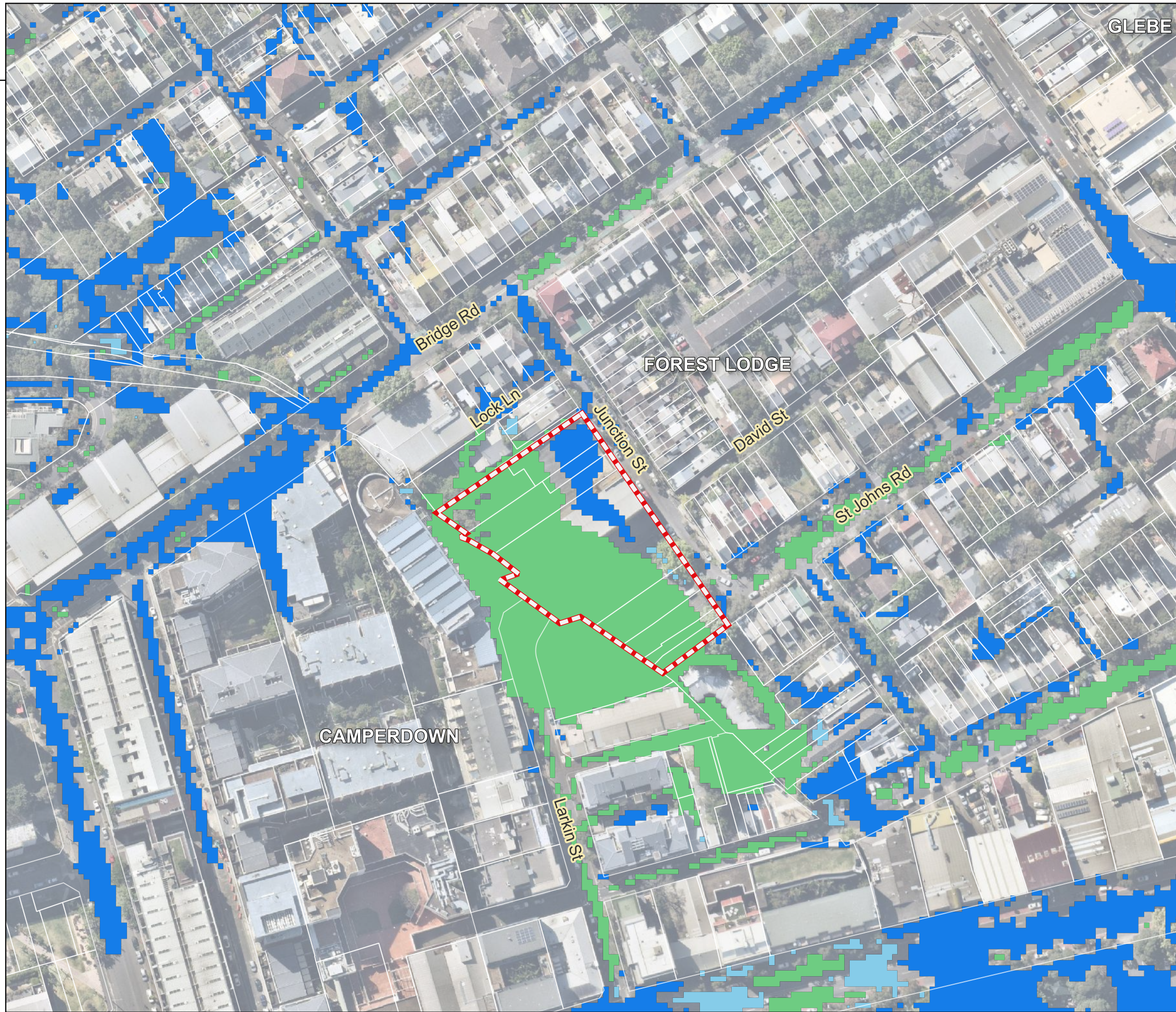
Figure 22 2% AEP Existing Peak Hazard
