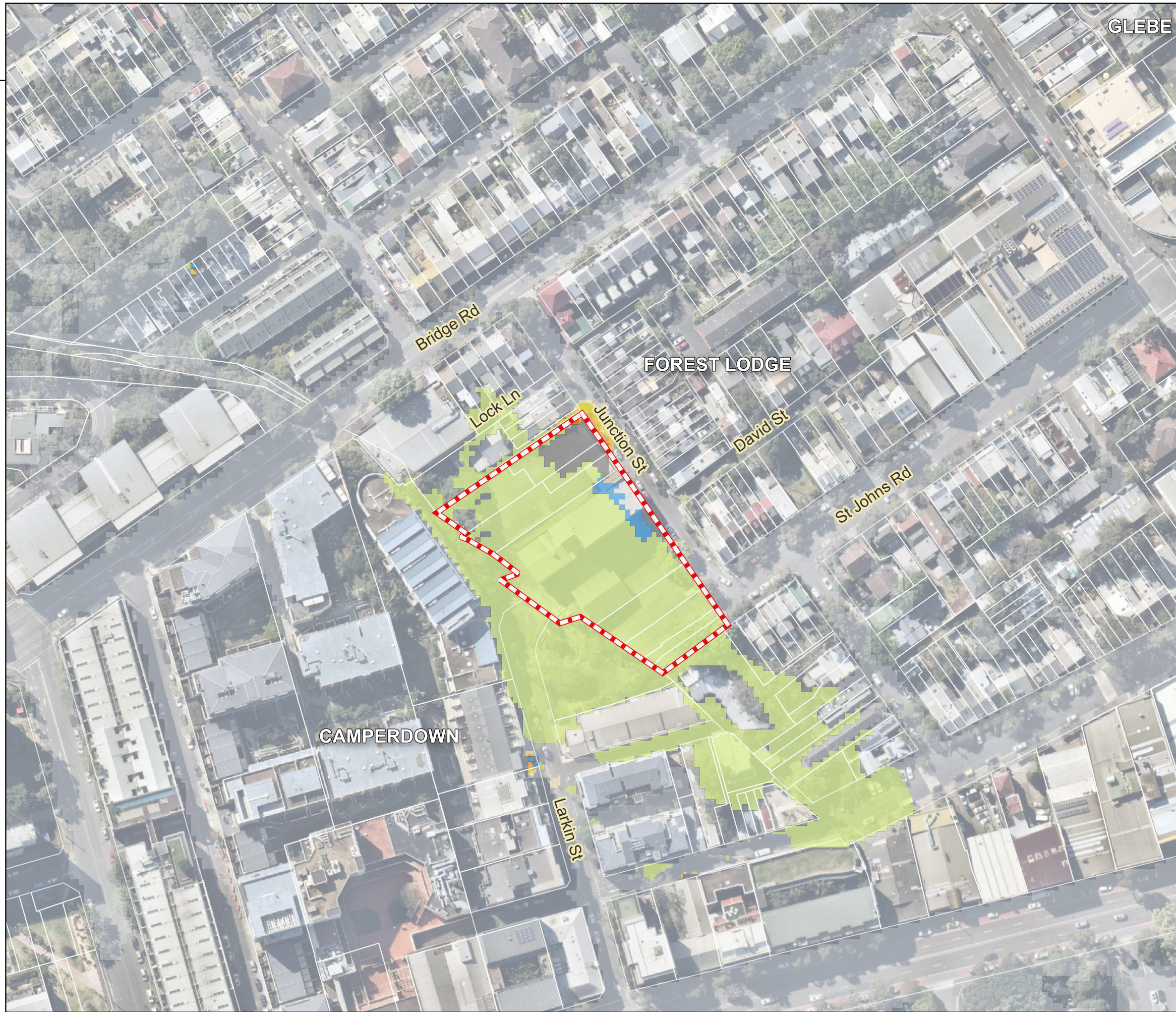
2-32 Junction Street Flood Impact Assessment Figure 58 2% AEP Change in Water Level (Post-Development less Existing)
