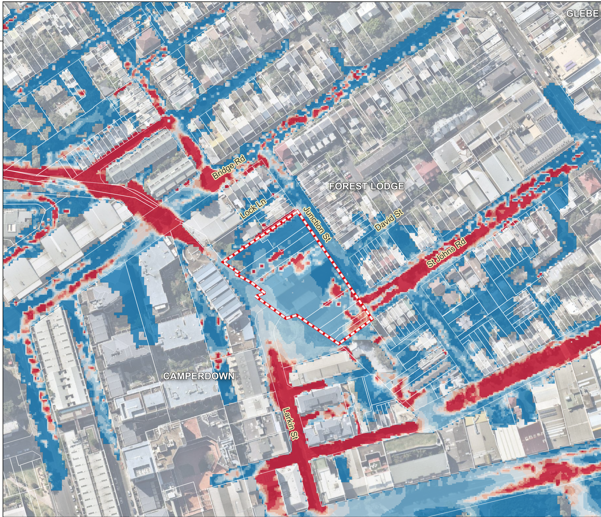
2-32 Junction Street Flood Impact Assessment Figure 43 PMF Post-Development Peak Velocity
