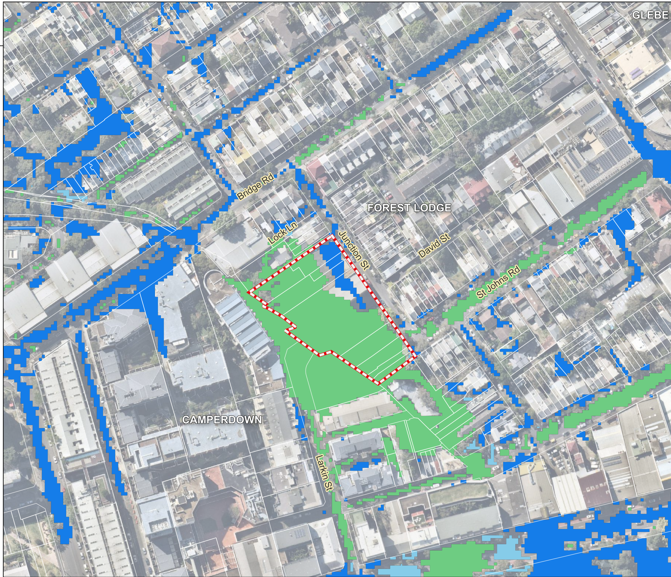
2-32 Junction Street Flood Impact Assessment Figure 27 1% AEP Sea Level Rise 0.9m Existing Peak Hazard
