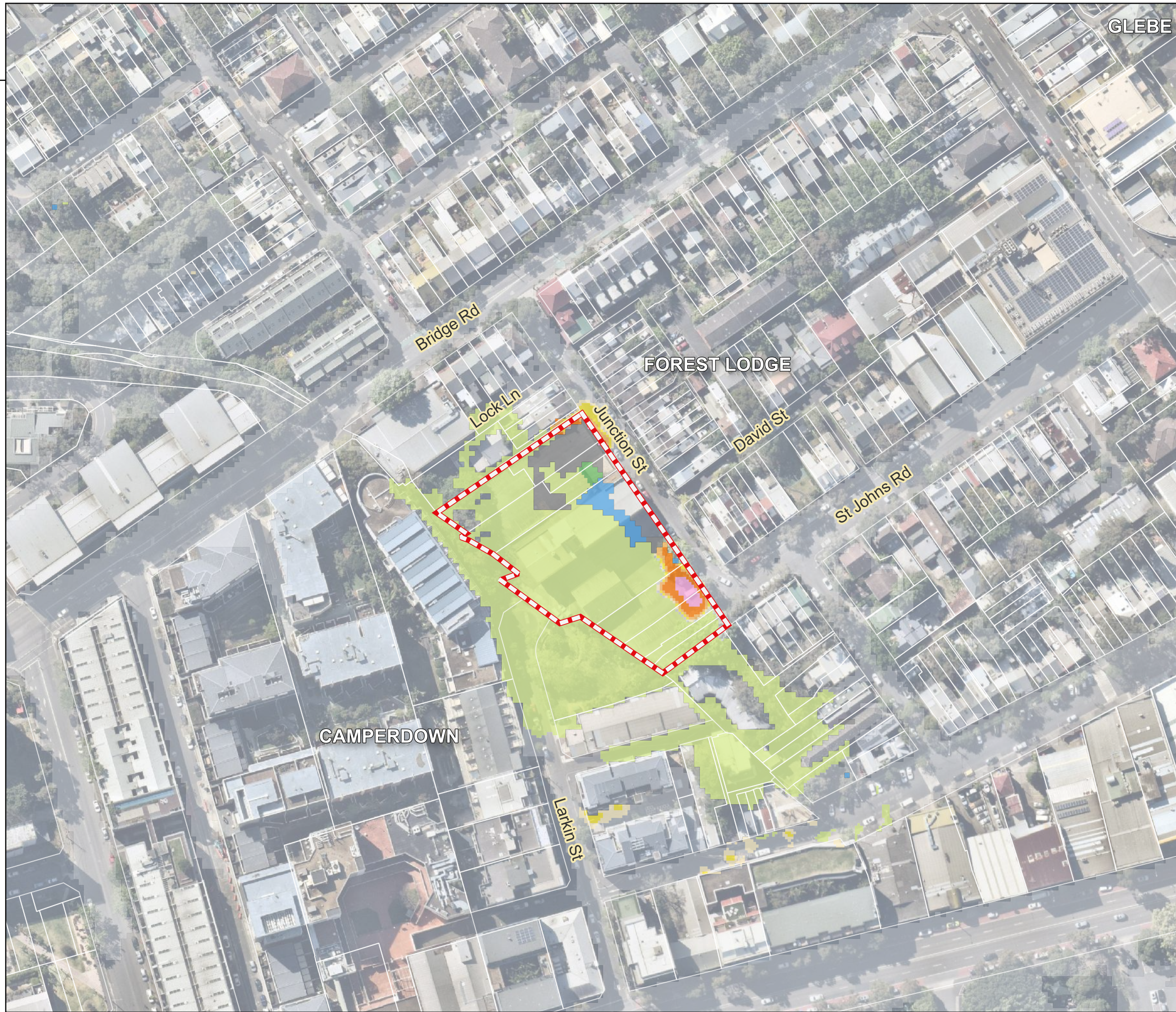
2-32 Junction Street Flood Impact Assessment Figure 57 5% AEP Change in Water Level (Post-Development less Existing)
