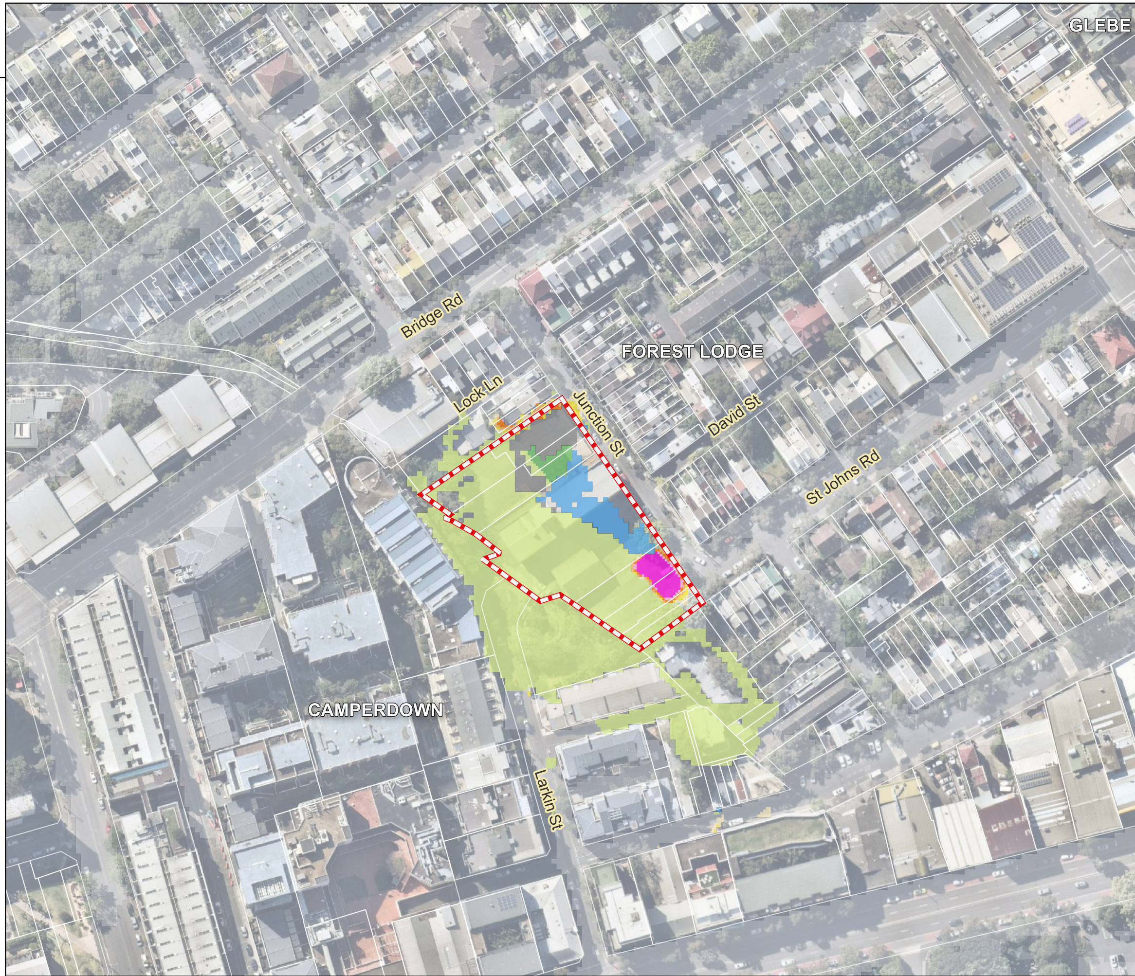
2-32 Junction Street Flood Impact Assessment Figure 55 20% AEP Change in Water Level (Post-Development less Existing)
