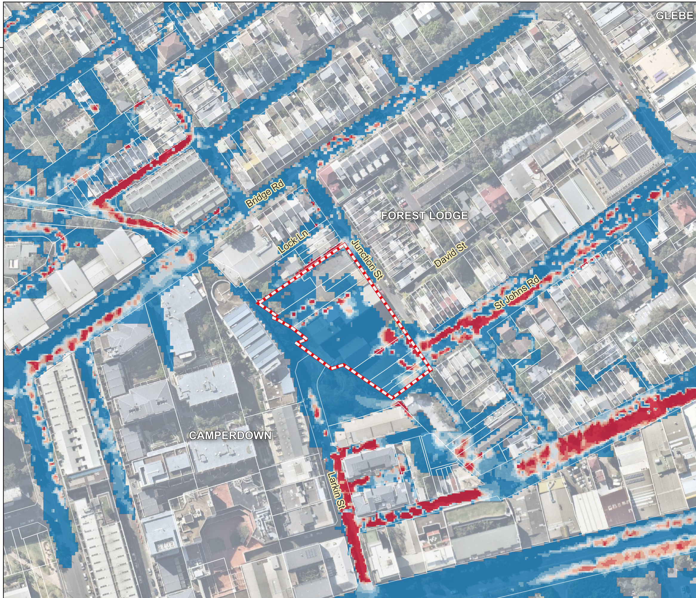
2-32 Junction Street Flood Impact Assessment Figure 39 5% AEP Post-Development Peak Velocity
