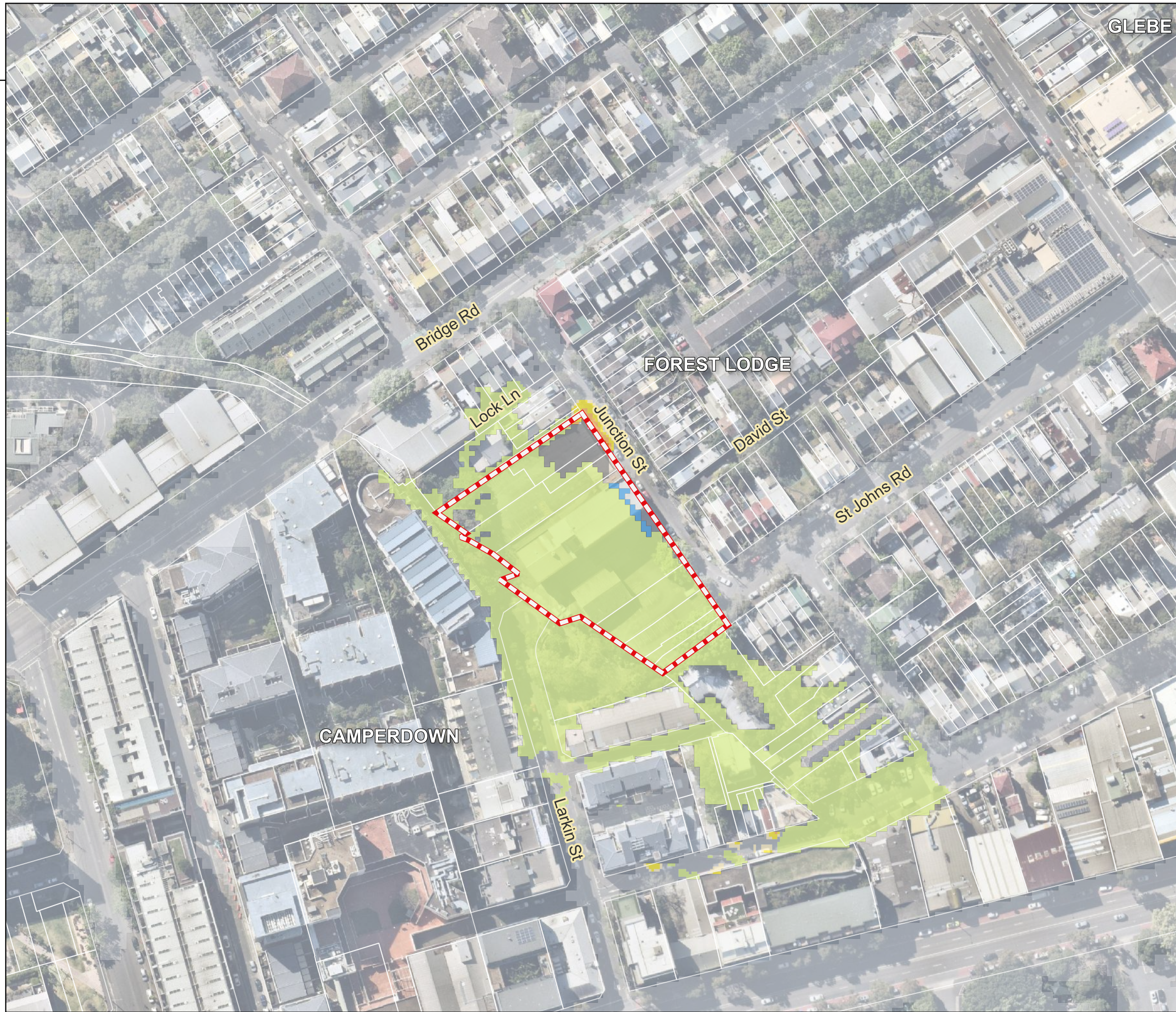
2-32 Junction Street Flood Impact Assessment Figure 62 1% AEP Sea Level Rise 0.4m Change in Water Level (Post-Development less Existing)
