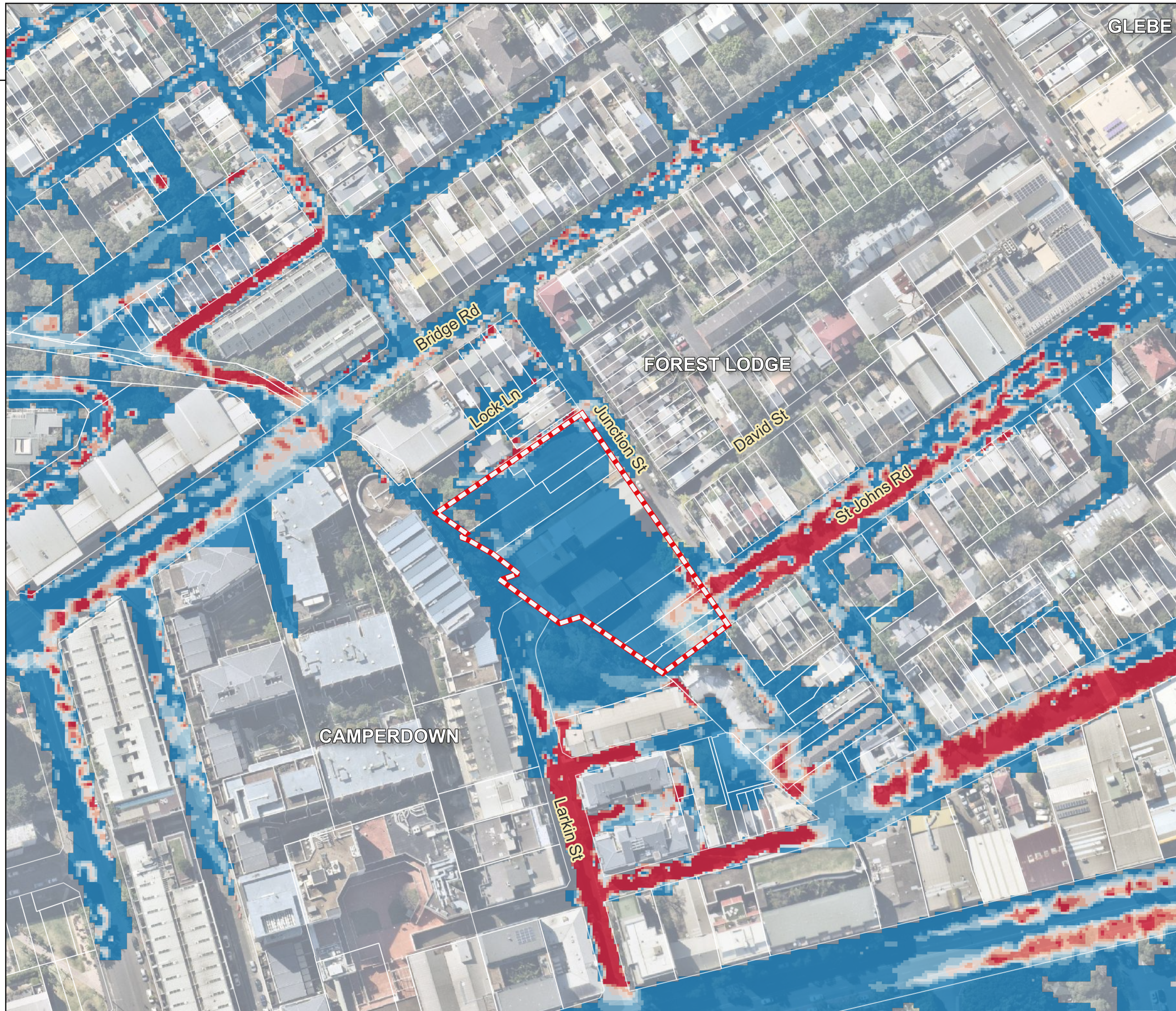
Figure 18 1% AEP Sea Level Rise 0.9m Existing Peak Velocity
