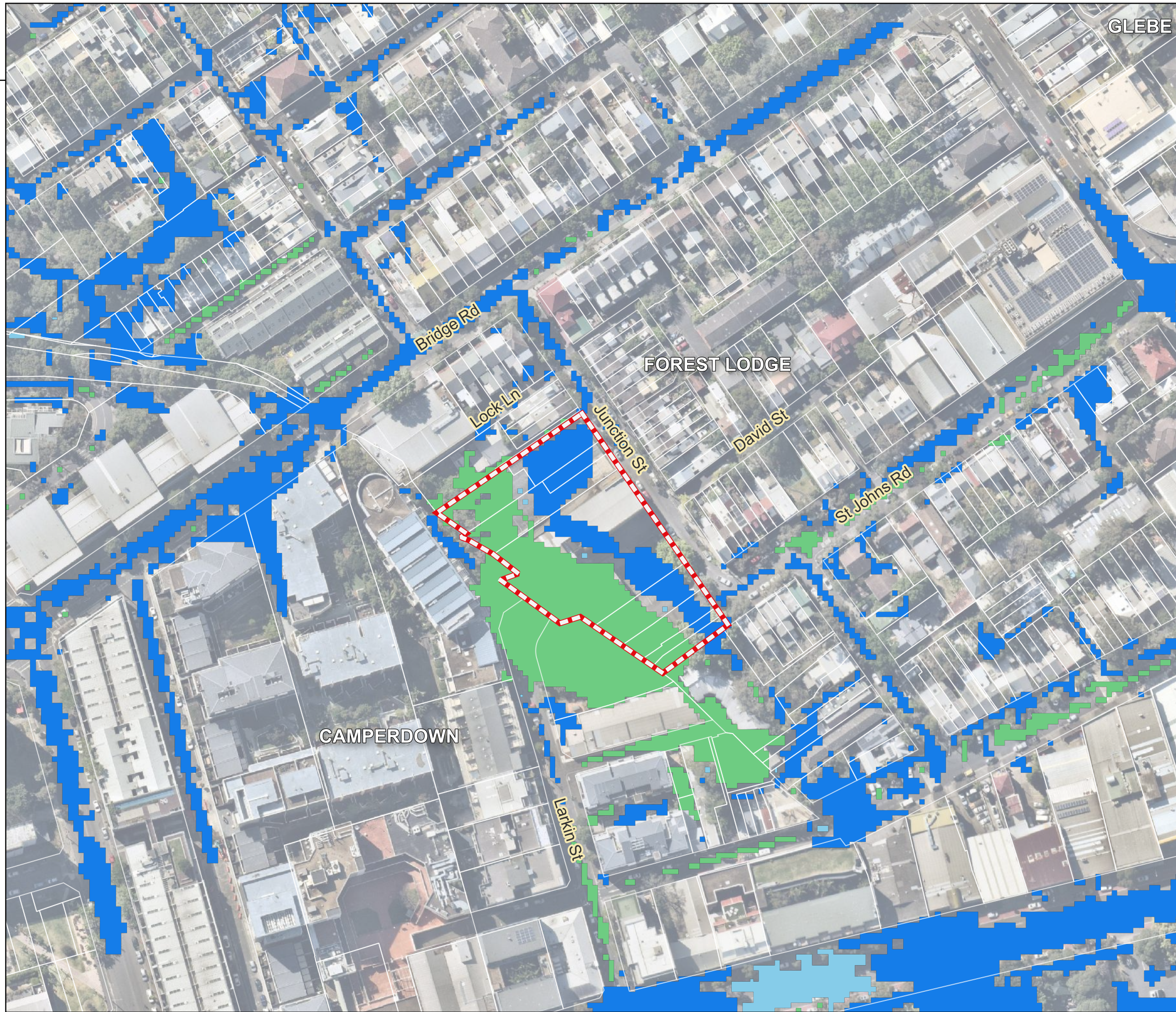
2-32 Junction Street Flood Impact Assessment Figure 20 10% AEP Existing Peak Hazard
