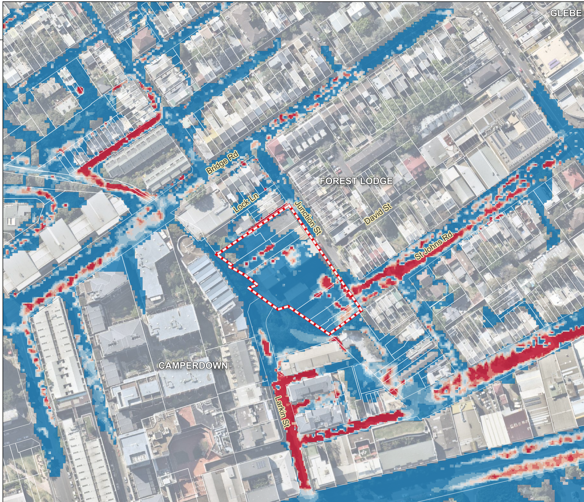
2-32 Junction Street Flood Impact Assessment Figure 40 2% AEP Post-Development Peak Velocity
