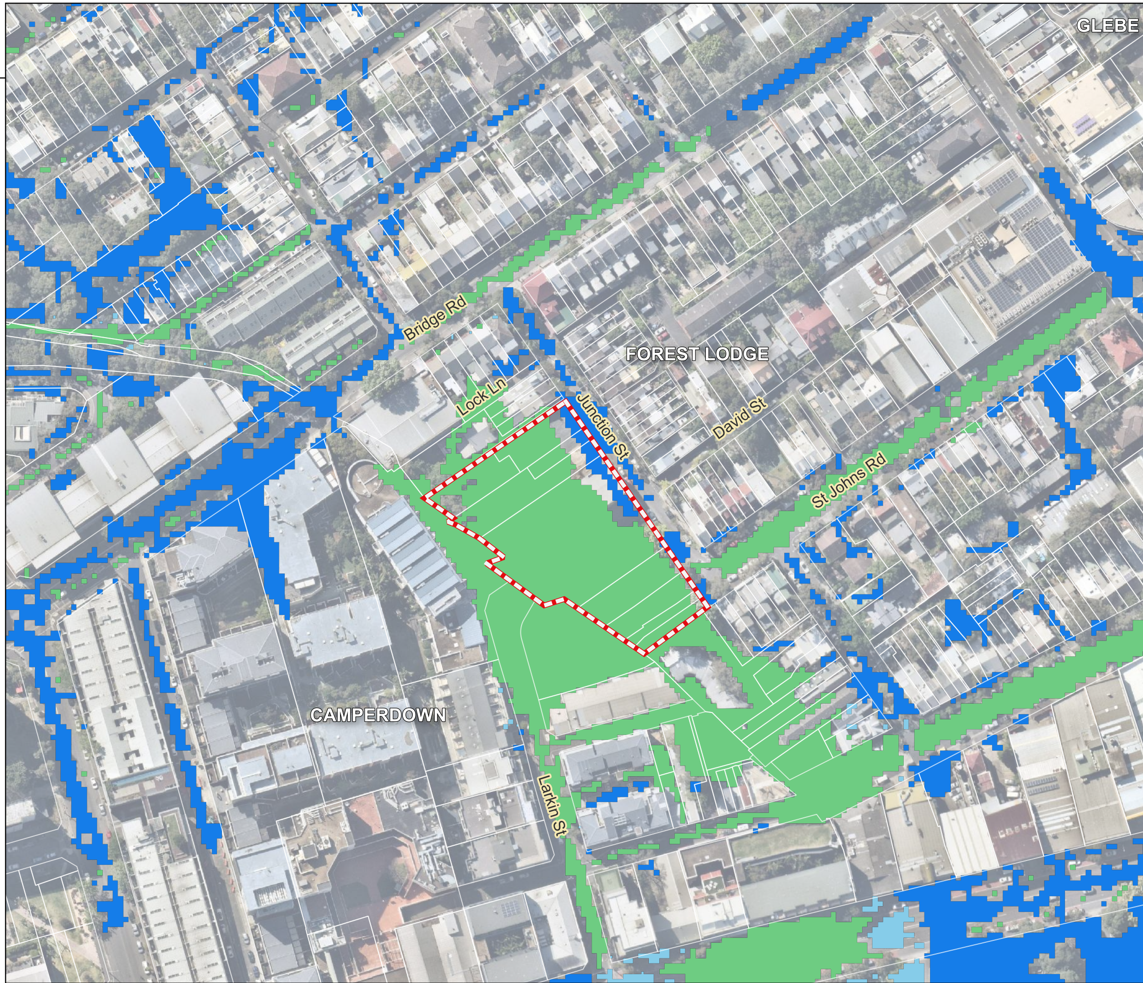
2-32 Junction Street Flood Impact Assessment Figure 24 0.2% AEP Existing Peak Hazard
