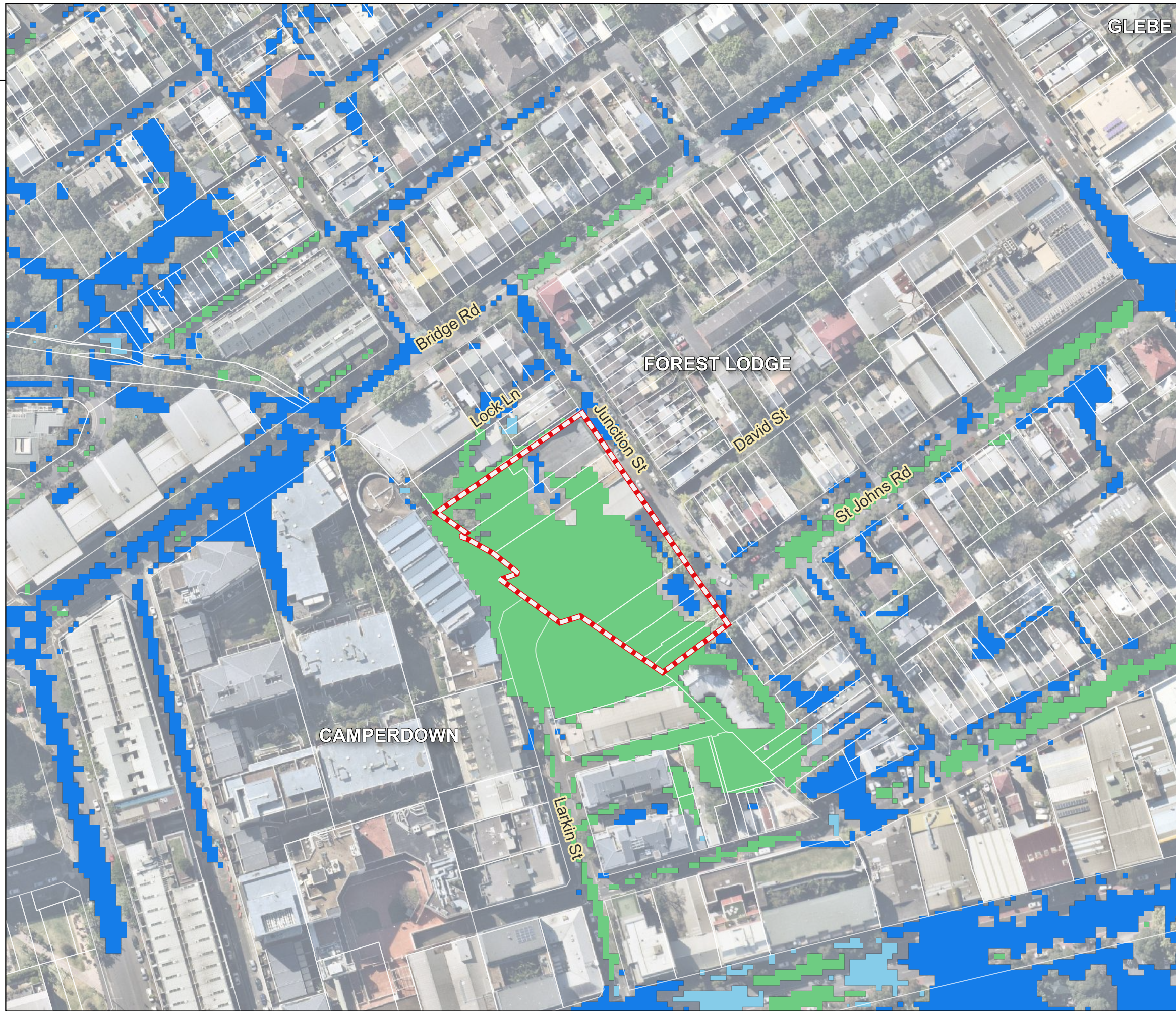
2-32 Junction Street Flood Impact Assessment Figure 49 2% AEP Post-Development Peak Hazard
