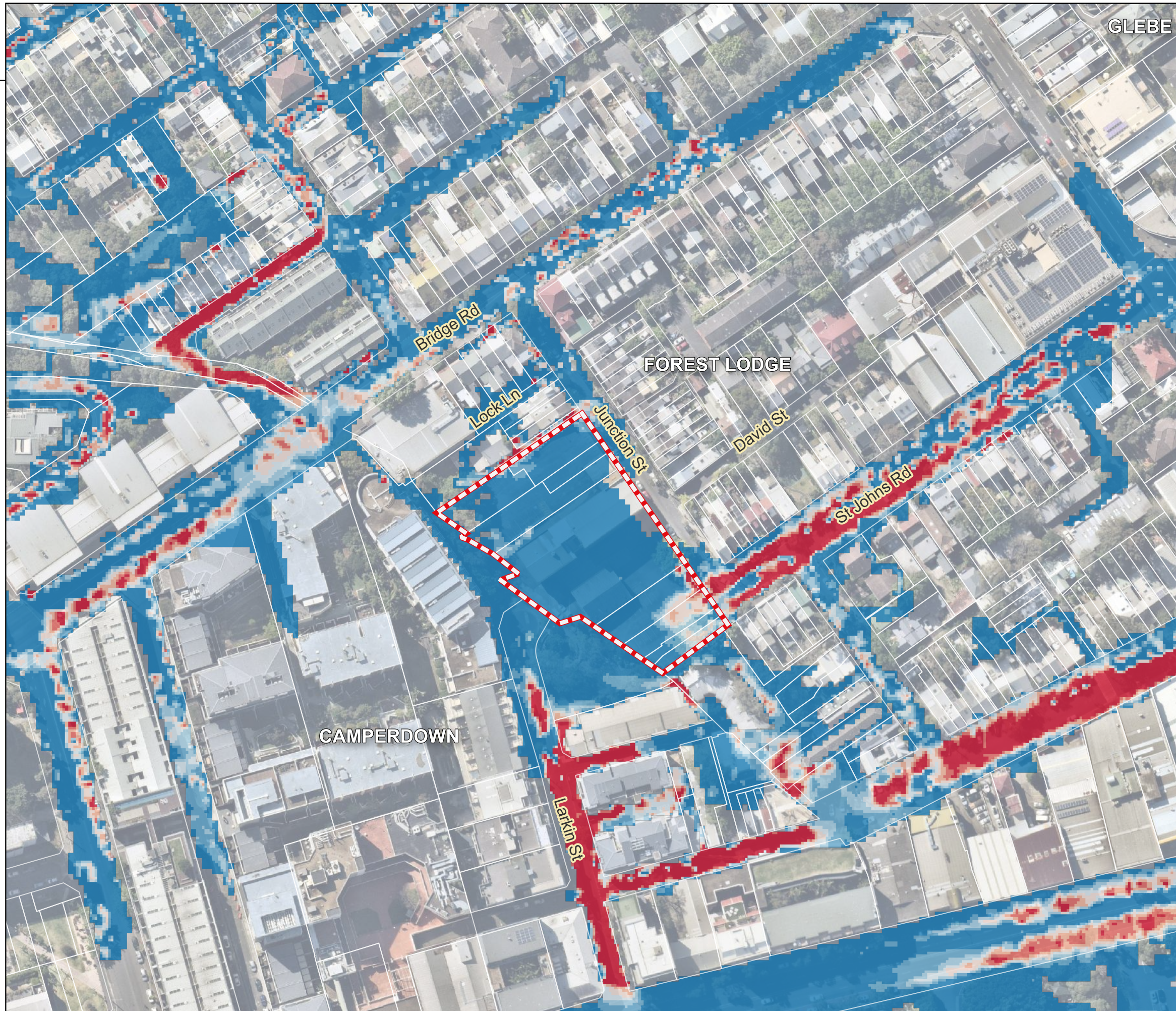
Figure 14 1% AEP Existing Peak Velocity
