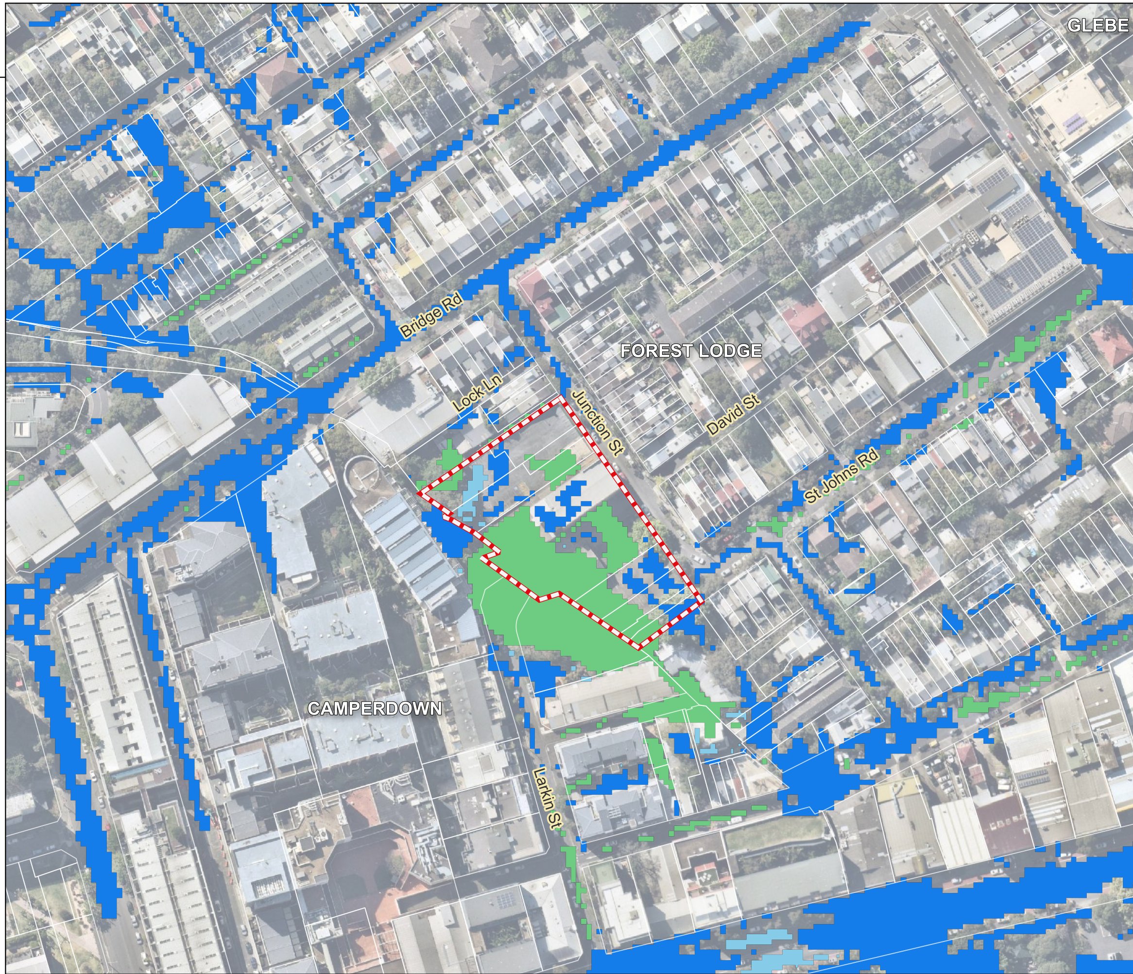
2-32 Junction Street Flood Impact Assessment Figure 46 20% AEP Post-Development Peak Hazard
