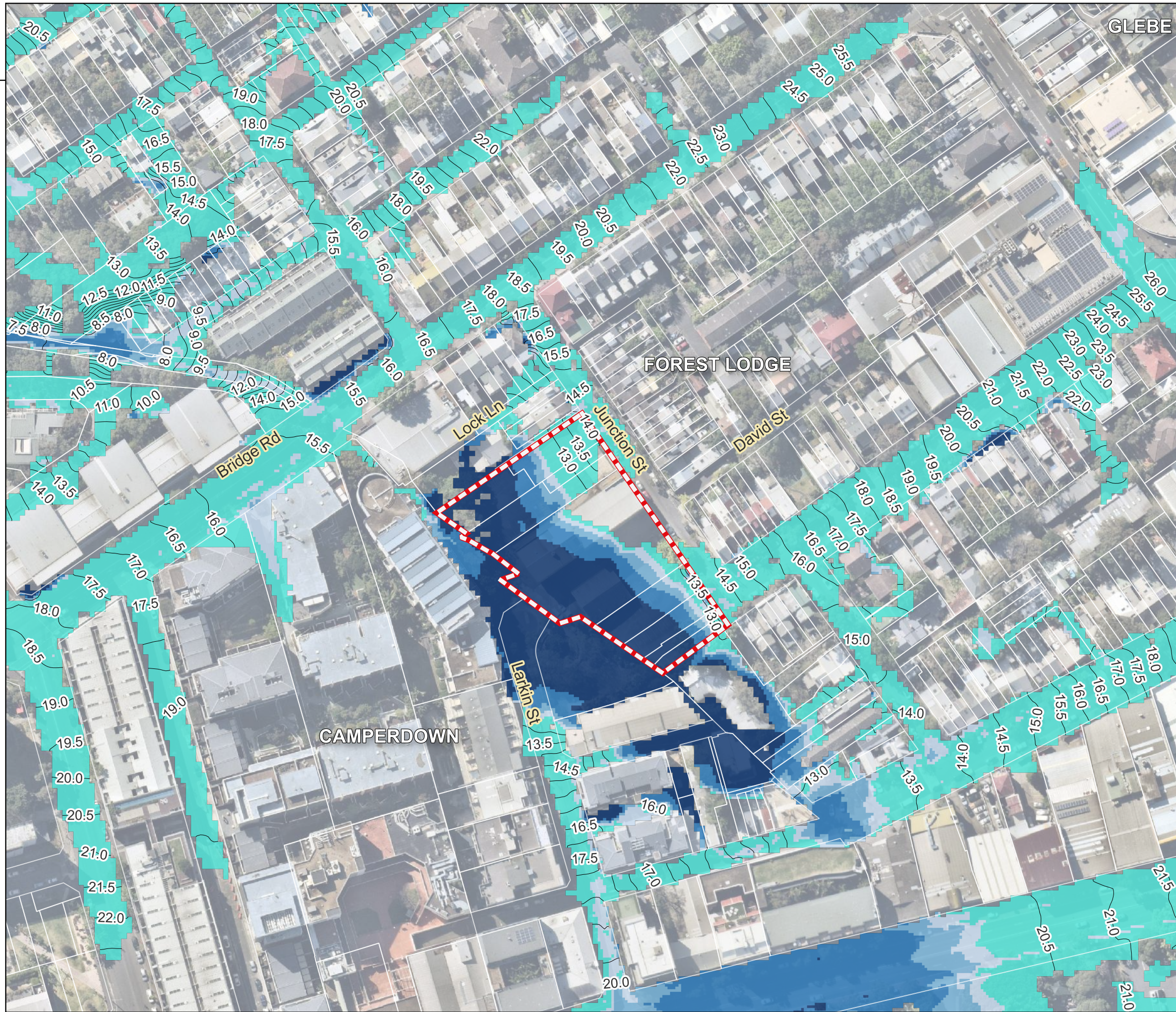
2-32 Junction Street Flood Impact Assessment Figure 02 10% AEP Existing Peak Depth and Water Level Contours
