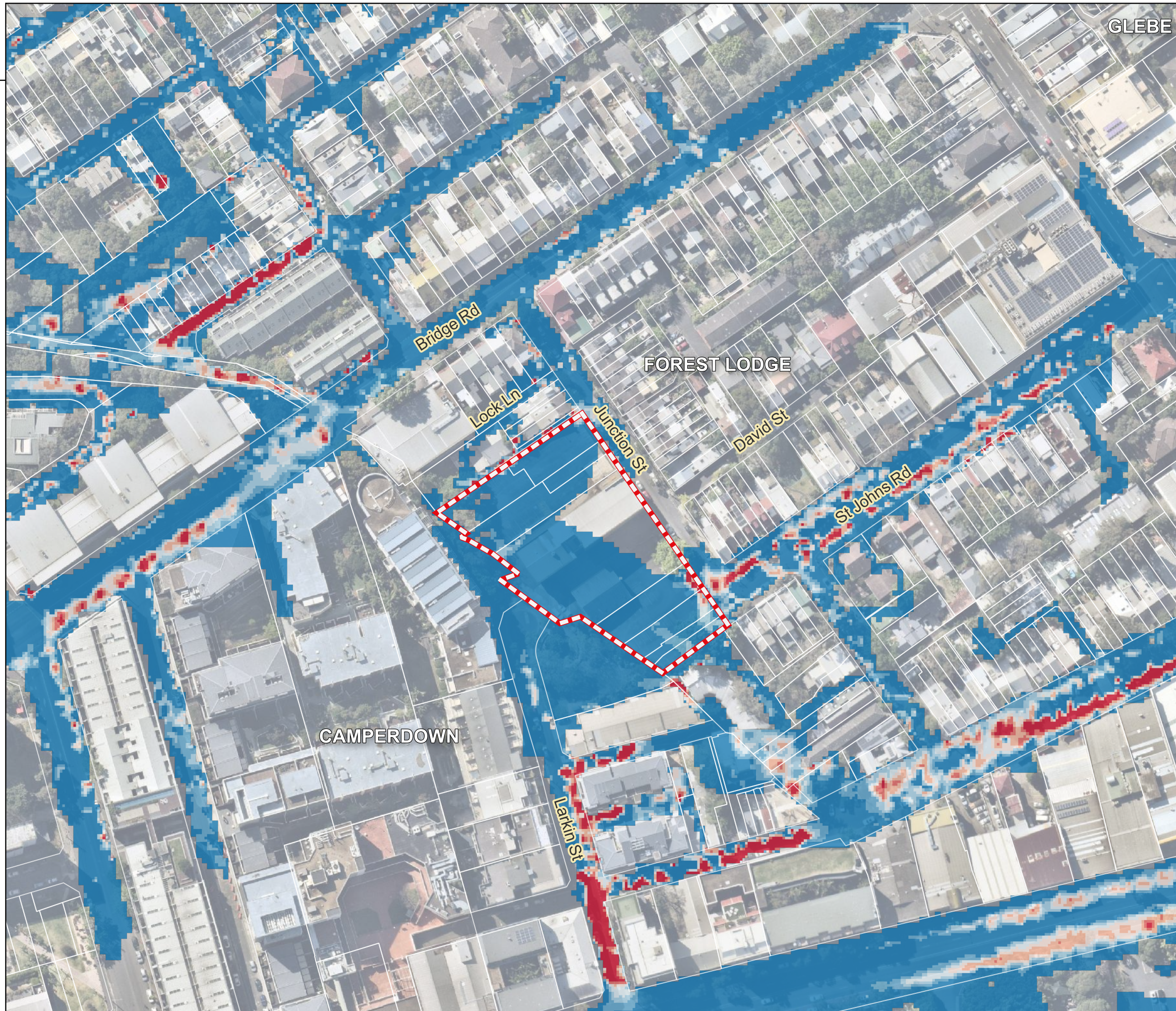
2-32 Junction Street Flood Impact Assessment Figure 10 20% AEP Existing Peak Velocity
