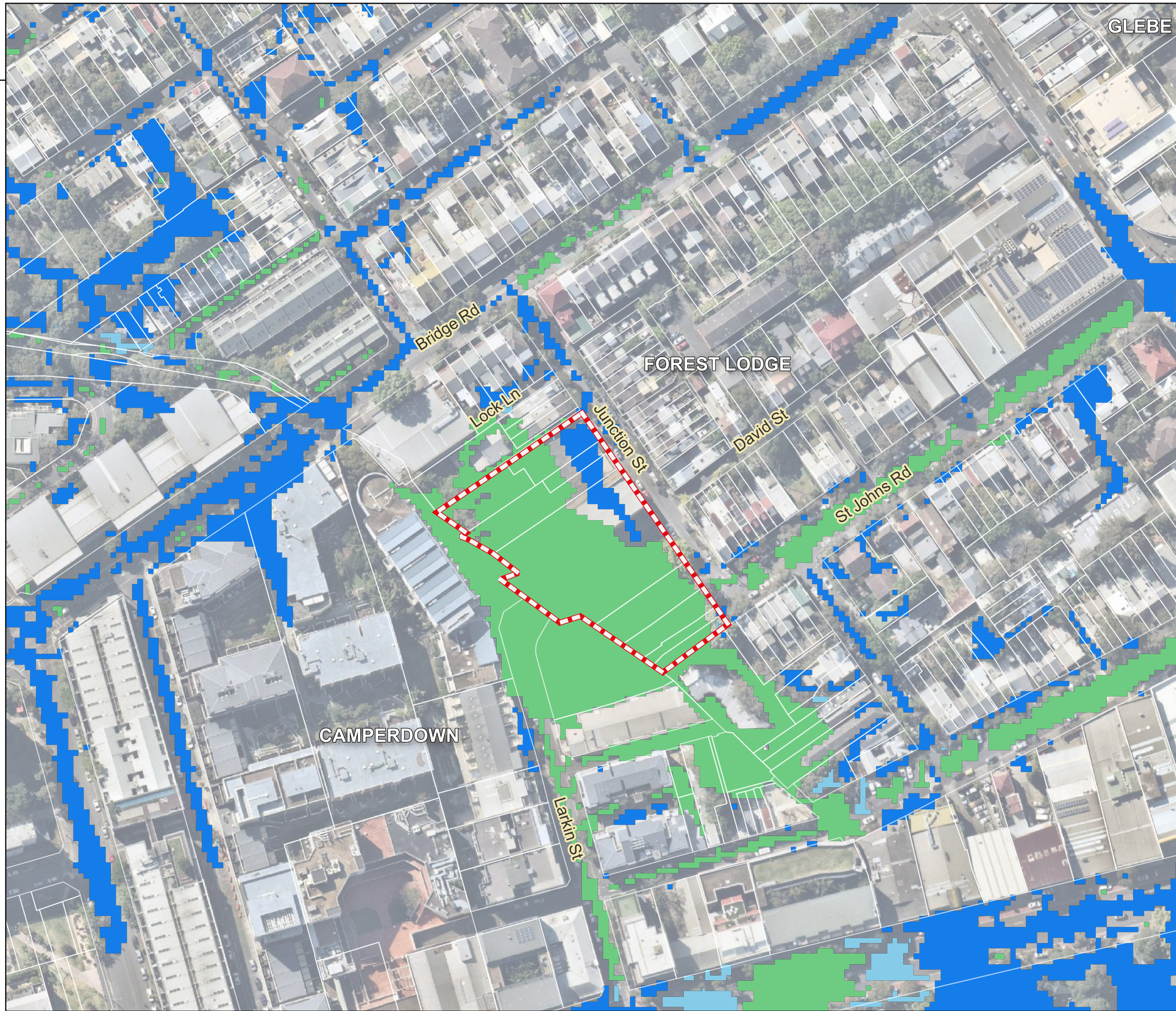
2-32 Junction Street Flood Impact Assessment Figure 23 1% AEP Existing Peak Hazard
