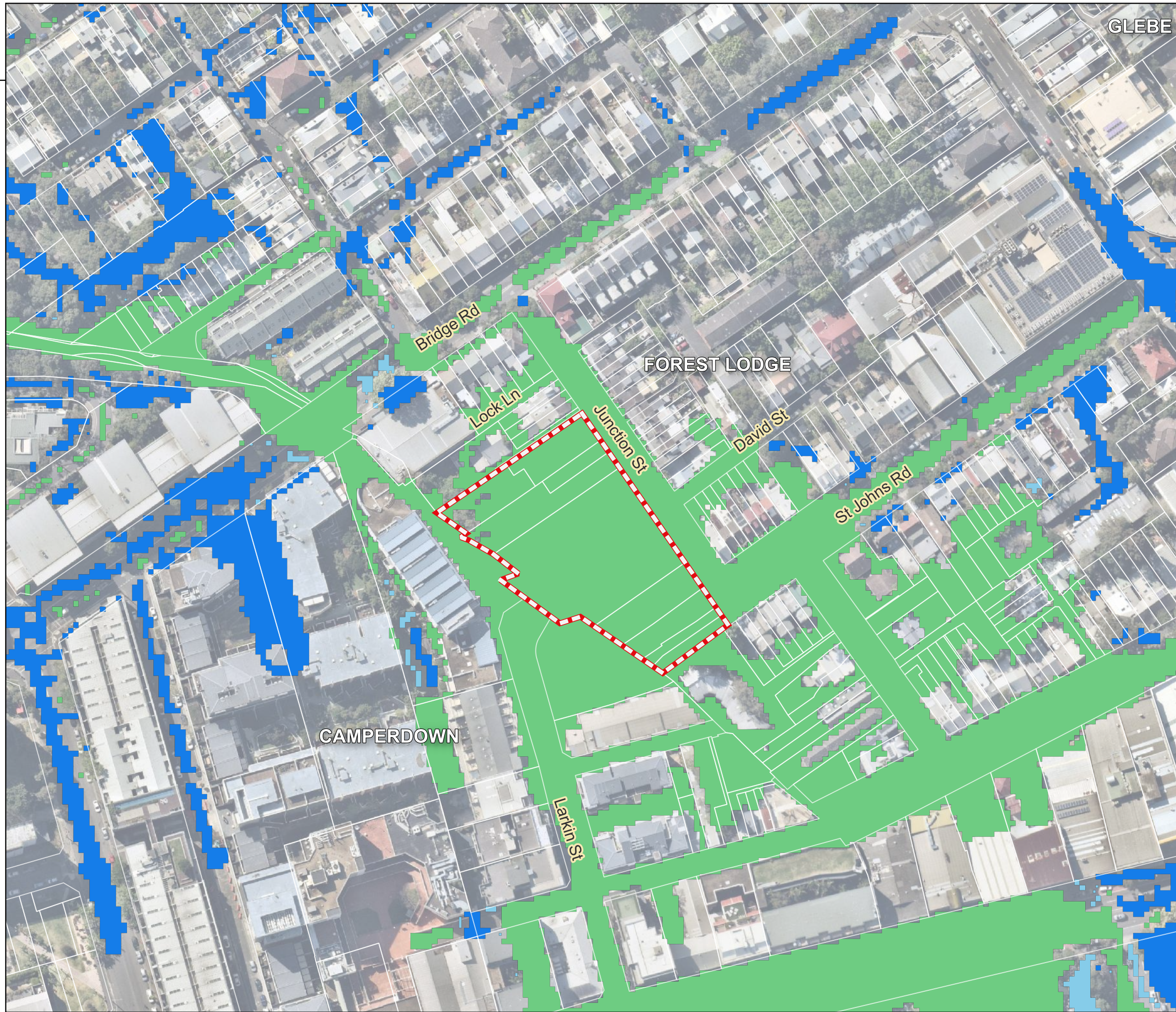
2-32 Junction Street Flood Impact Assessment Figure 25 PMF Existing Peak Hazard
