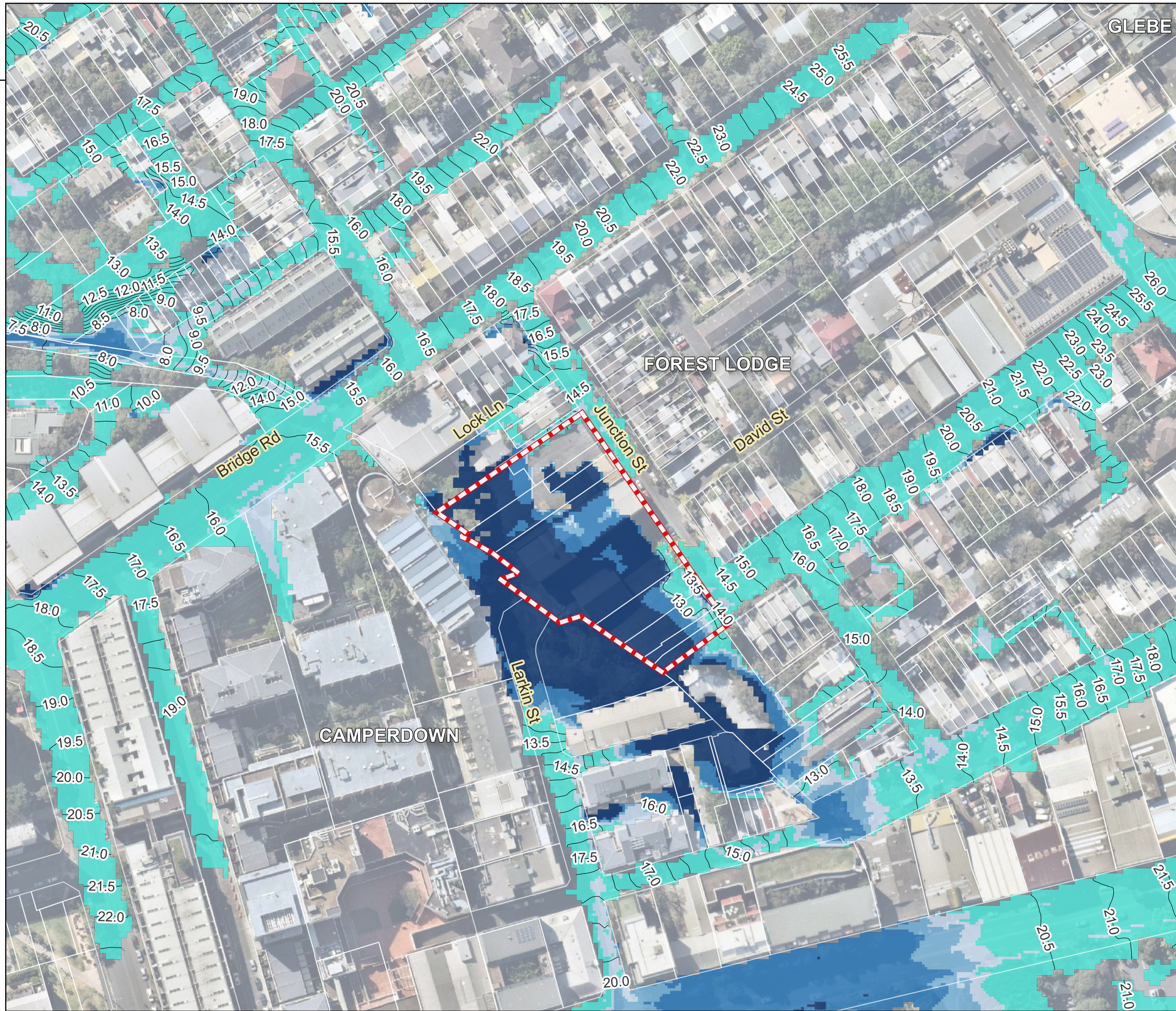
2-32 Junction Street Flood Impact Assessment Figure 29 10% AEP Post-Development Peak Depth and Water Level Contours
