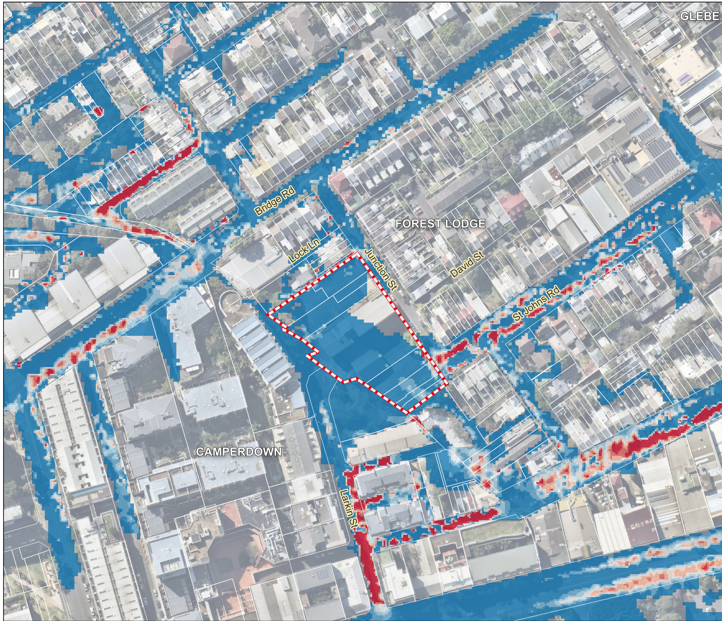
Figure 11 10% AEP Existing Peak Velocity
