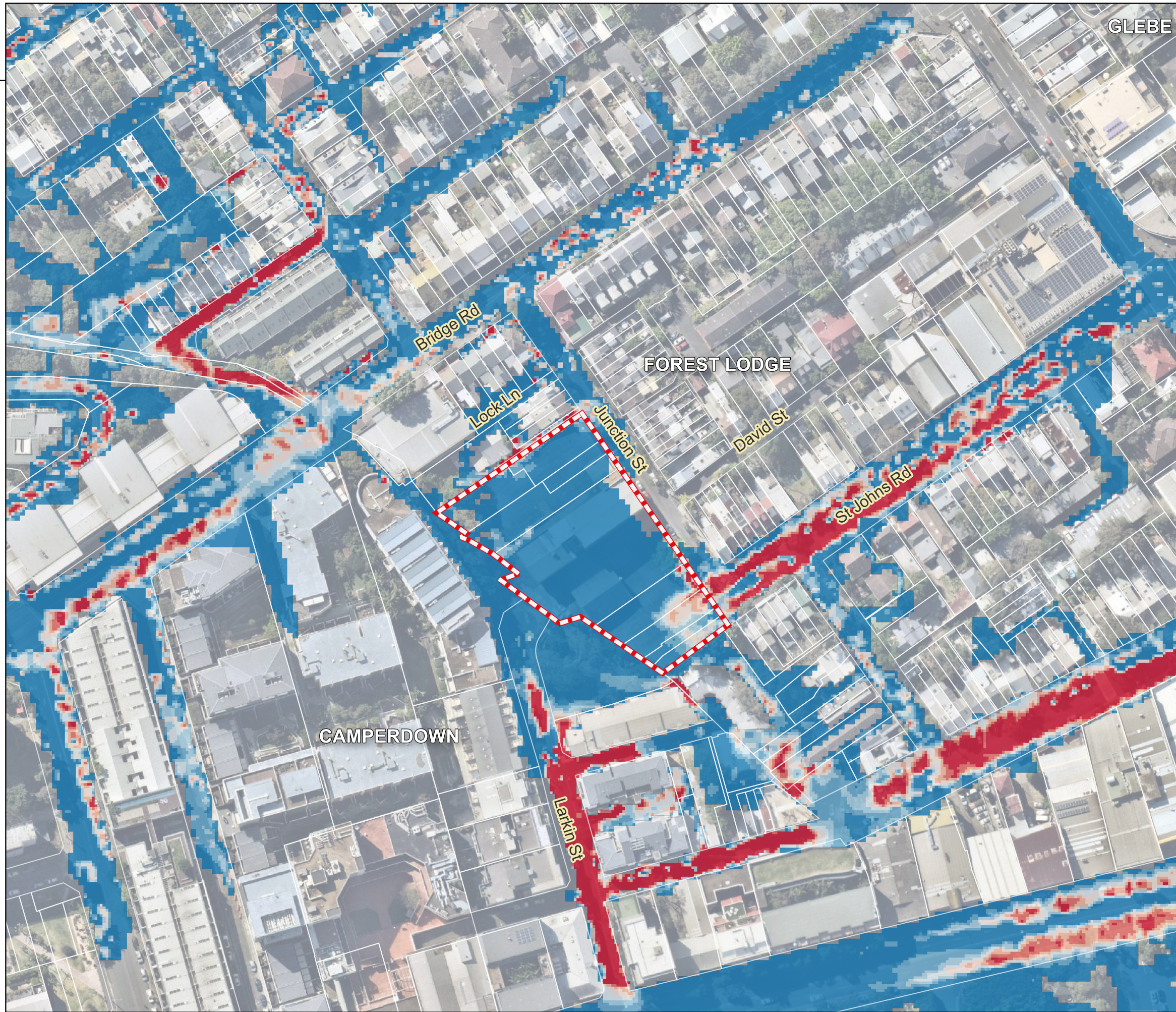
Figure 17 1% AEP Sea Level Rise 0.4m Existing Peak Velocity
