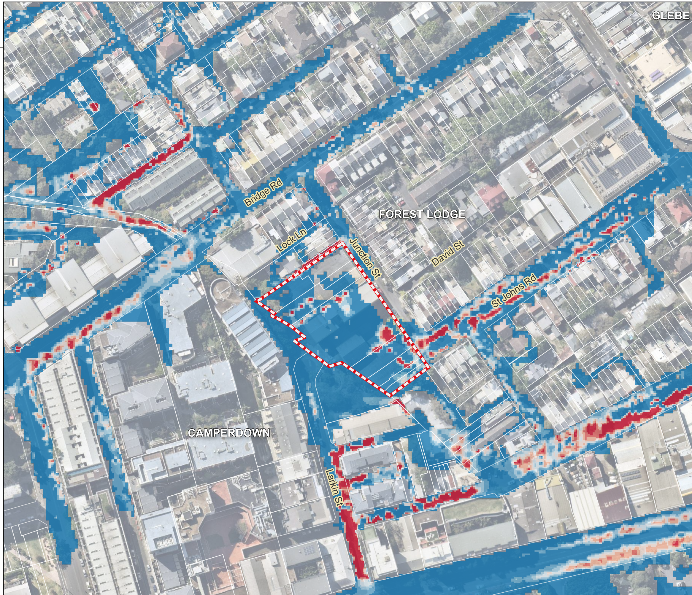
2-32 Junction Street Flood Impact Assessment Figure 38 10% AEP Post-Development Peak Velocity
