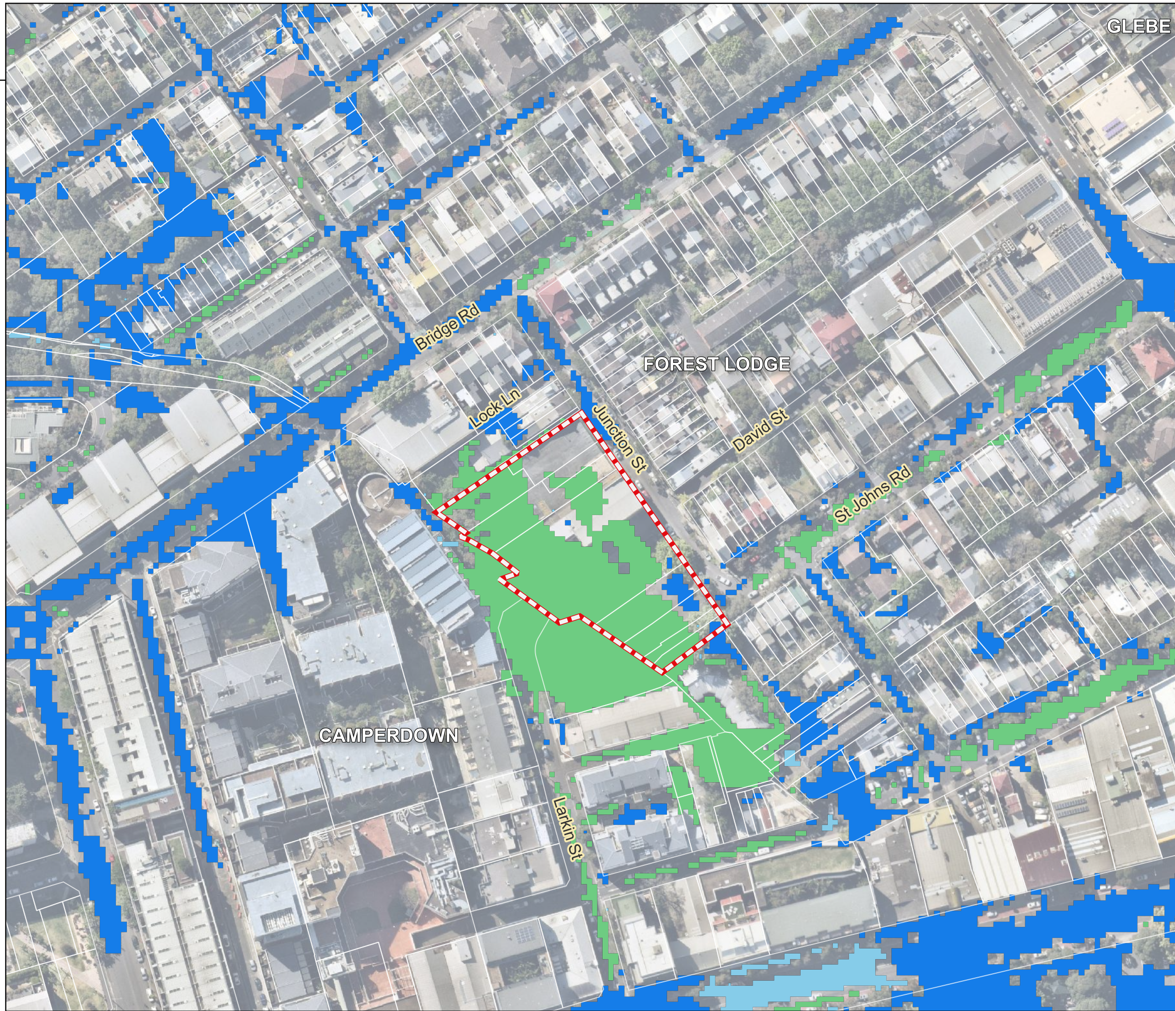
2-32 Junction Street Flood Impact Assessment Figure 48 5% AEP Post-Development Peak Hazard
