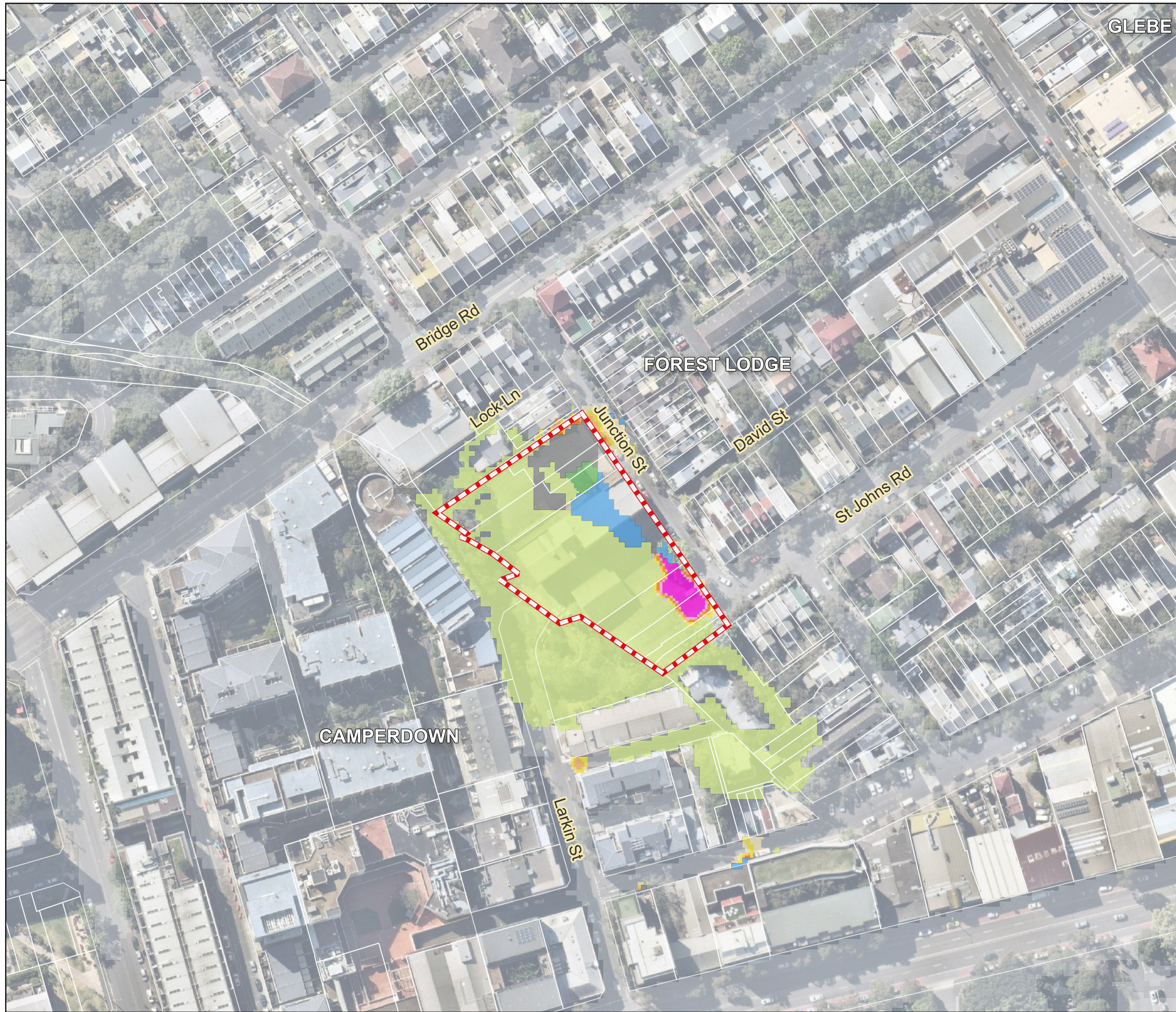
2-32 Junction Street Flood Impact Assessment Figure 56 10% AEP Change in Water Level (Post-Development less Existing)
