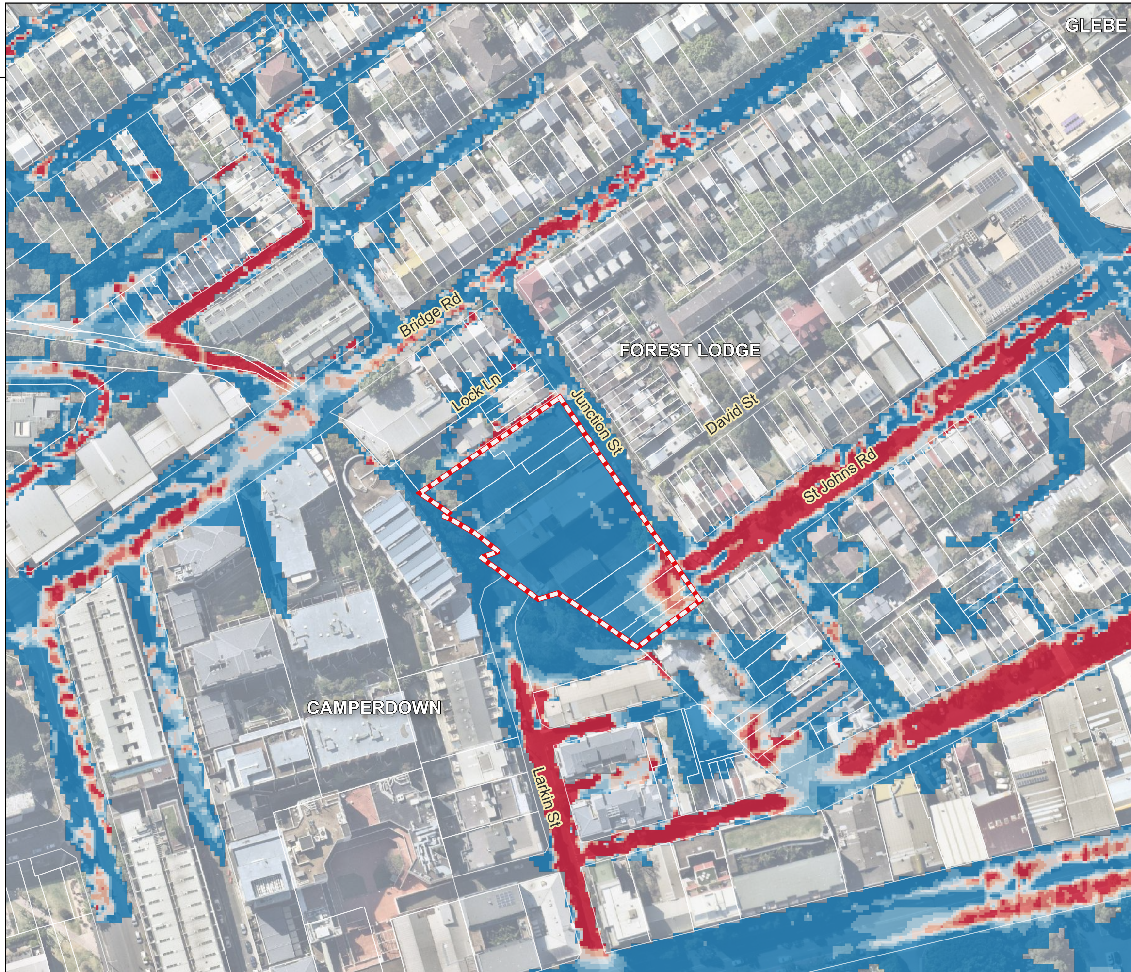
Figure 15 0.2% AEP Existing Peak Velocity
