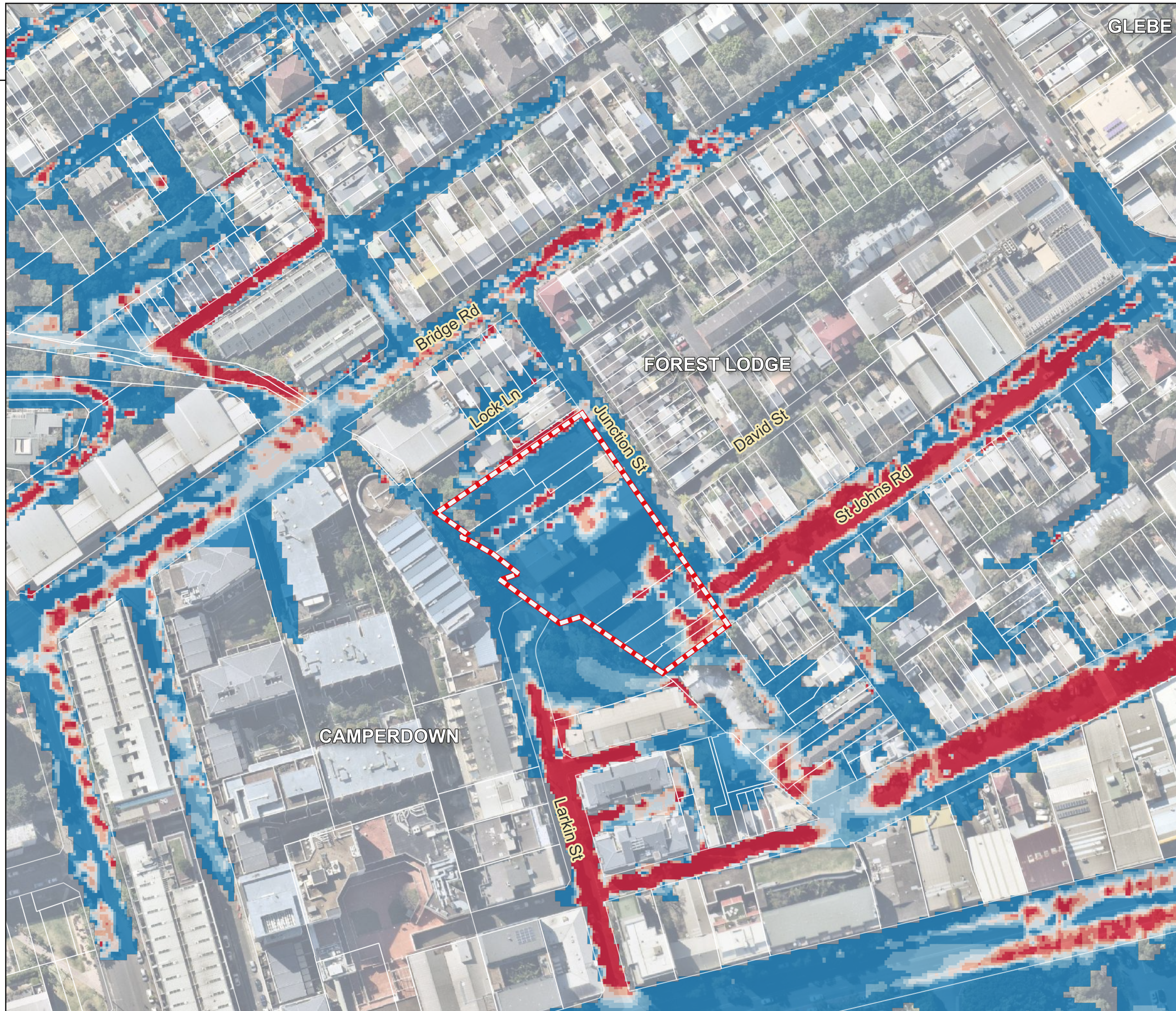
2-32 Junction Street Flood Impact Assessment Figure 42 0.2% AEP Post-Development Peak Velocity
