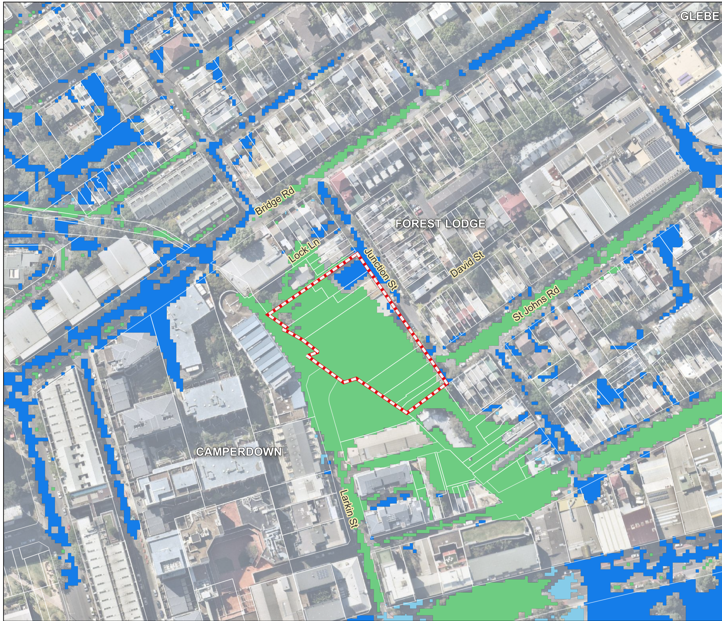
2-32 Junction Street Flood Impact Assessment Figure 51 0.2% AEP Post-Development Peak Hazard
