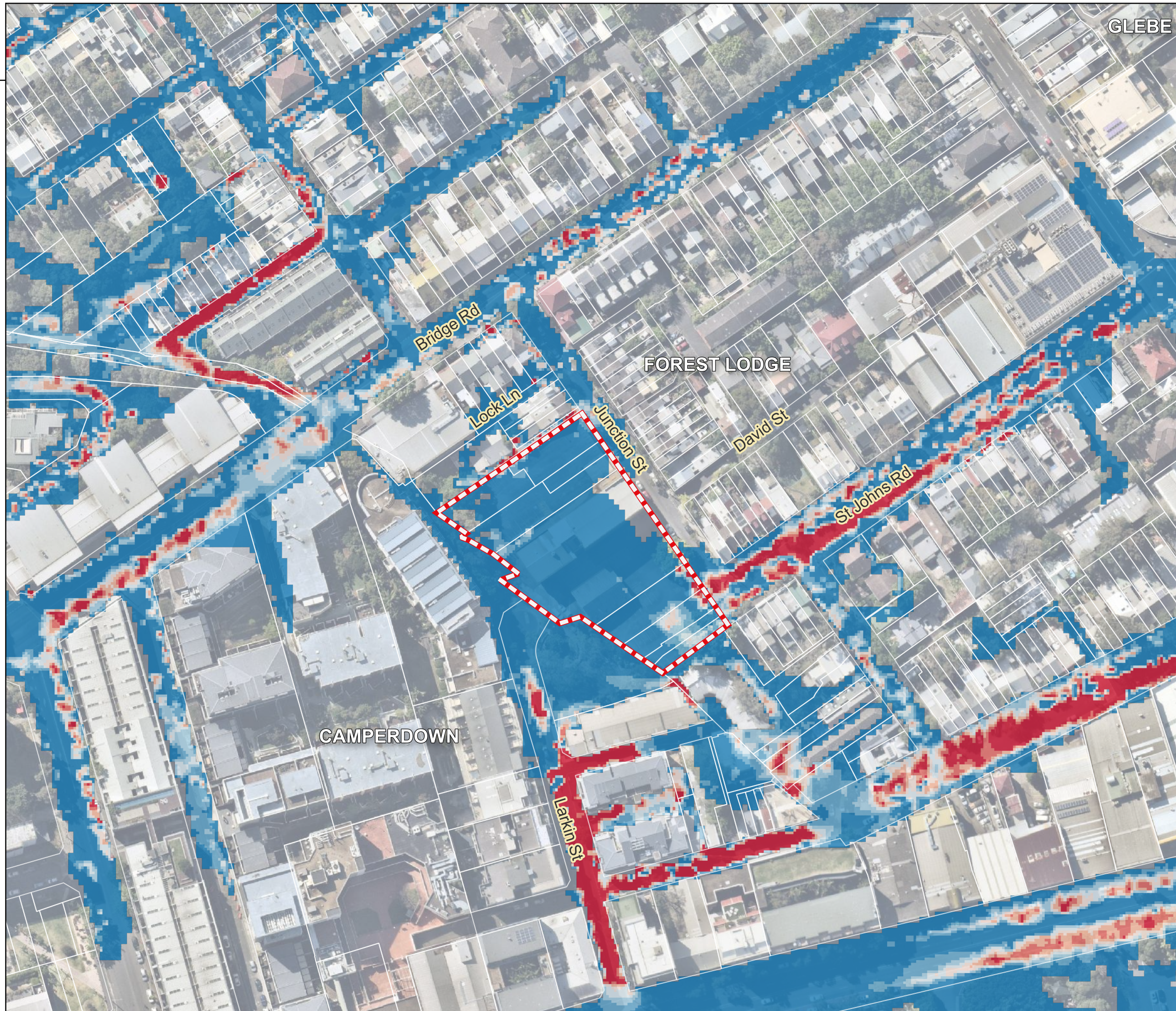
Figure 13 2% AEP Existing Peak Velocity
