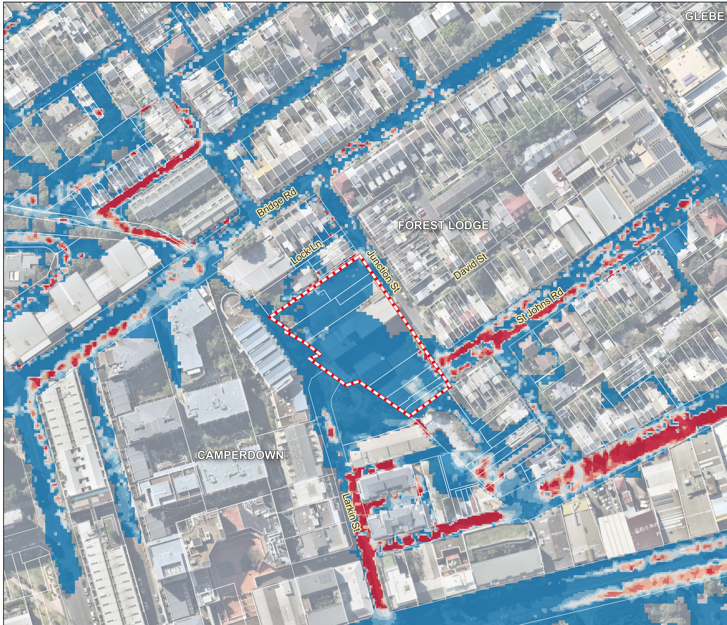
Figure 12 5% AEP Existing Peak Velocity
