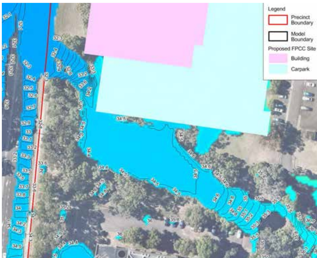
Figure 5-1 100yr ARI Peak Water Levels for Stage 1 Scenario – FPCC Site
