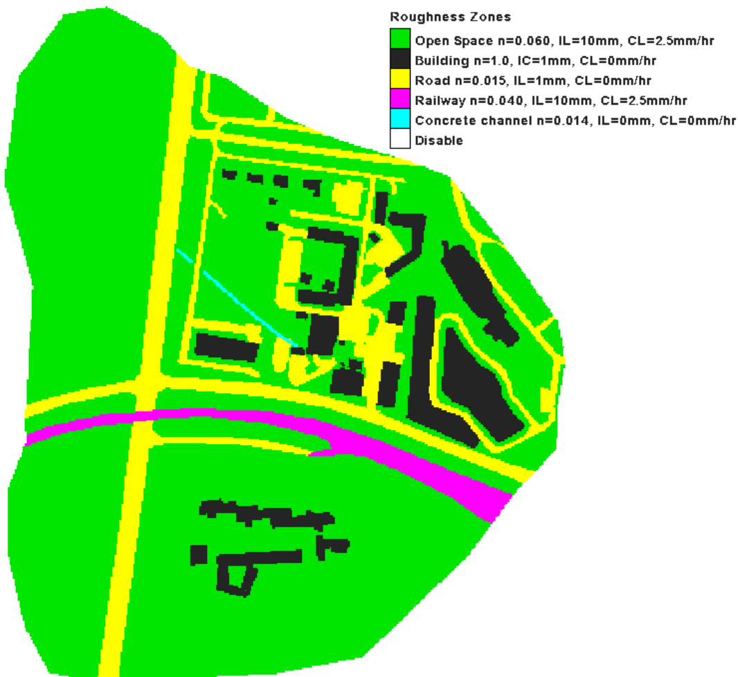
Figure 3-2 Land Use Breakdown for the Model Area
