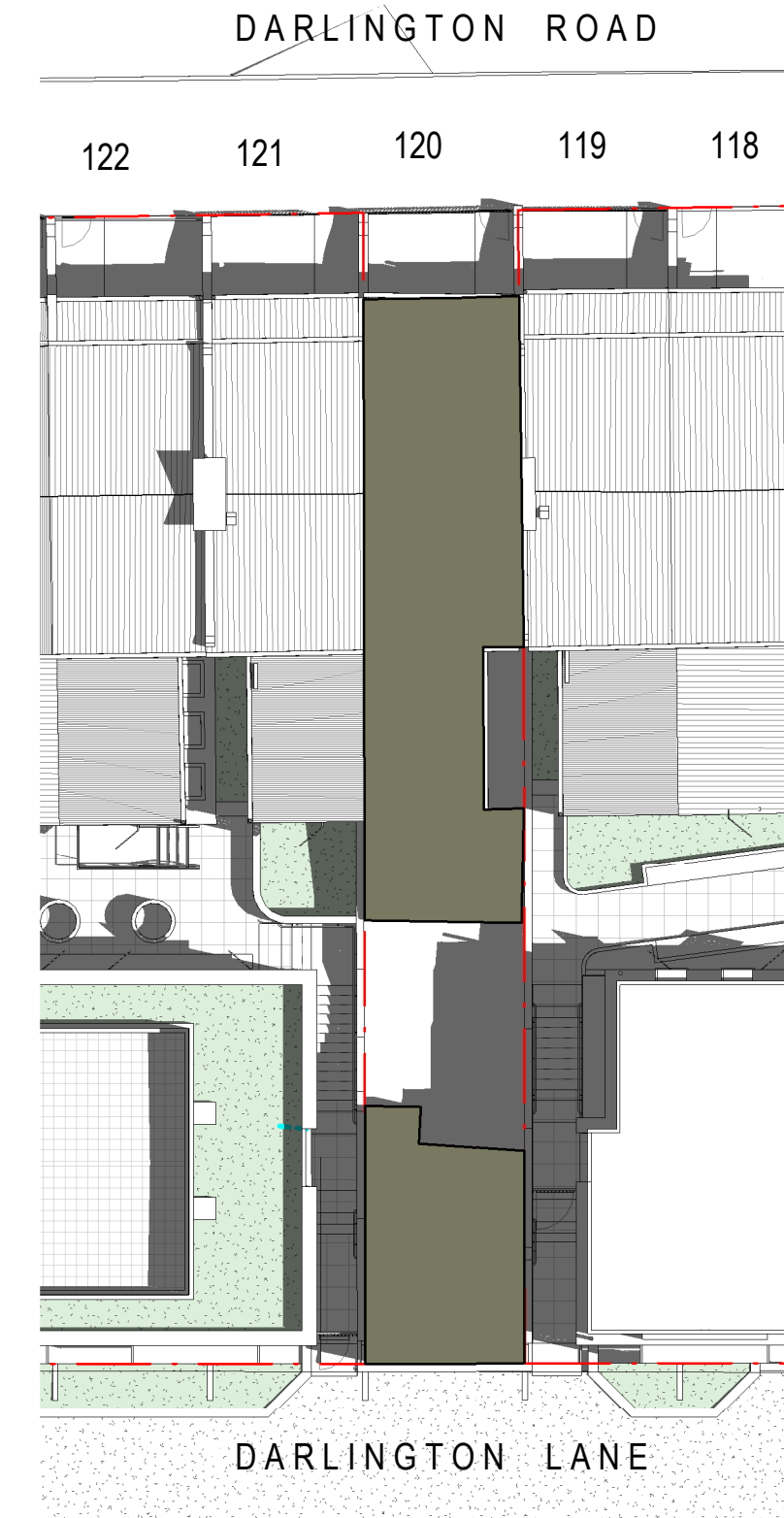
11 15 DECEMBER 9.30AM 1:200 BETWEEN 9.30AM - 2.30PM (INCLUSIVE) NO.120 DARLINGTON ROAD RECEIVES 5 HOURS OF SOLAR ACCESS TO AT LEAST 8SQM OF THEIR REAR PRIVATE OPEN SPACE. 3 HOURS ABOVE THE SYDNEY DCP REQUIREMENT OF MIN. 2 HOURS
