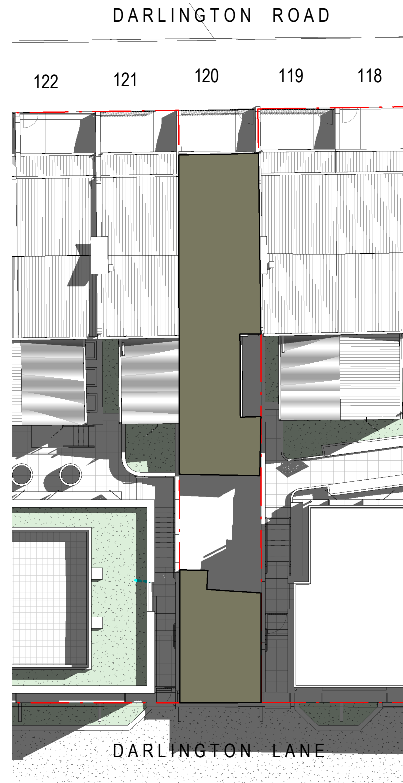
11 15 MARCH 10.30AM 1:200 BETWEEN 10.30AM - 2PM (INCLUSIVE) NO.120 DARLINGTON ROAD RECEIVES 3.5 HOURS OF SOLAR ACCESS TO AT LEAST 8SQM OF THEIR REAR PRIVATE OPEN SPACE. 1.5 HOURS ABOVE THE SYDNEY DCP REQUIREMENT OF MIN. 2 HOURS
