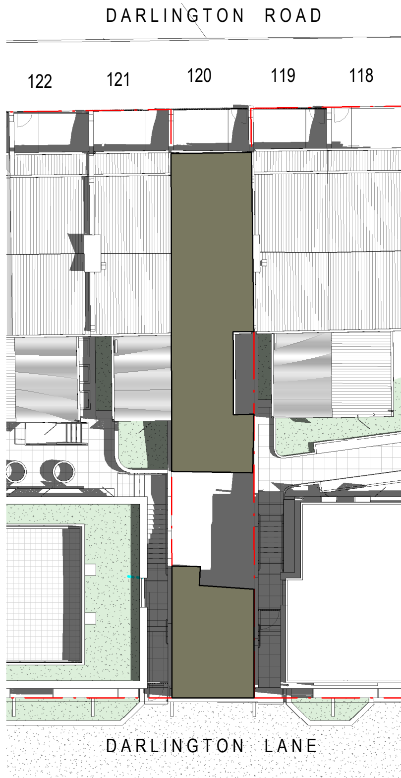
3 15 JANUARY 10AM 1:200 BETWEEN 10AM - 3PM (INCLUSIVE) NO.120 DARLINGTON ROAD RECEIVES 5 HOURS OF SOLAR ACCESS TO AT LEAST 8SQM OF THEIR REAR PRIVATE OPEN SPACE. 3 HOURS ABOVE THE SYDNEY DCP REQUIREMENT OF MIN. 2 HOURS
