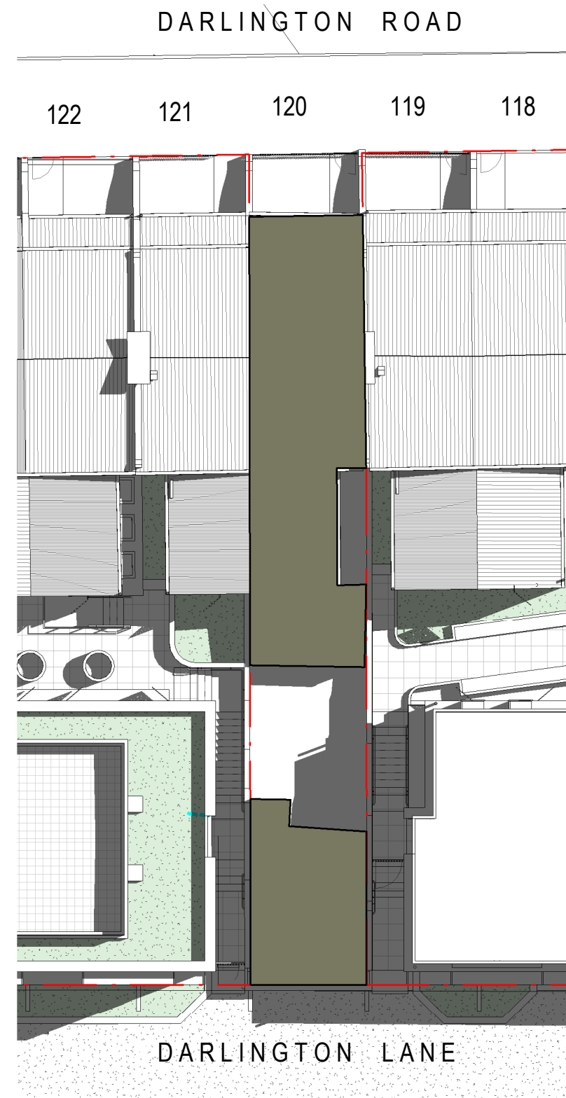
9 01 MARCH 10.30AM 1:200 BETWEEN 10.30AM - 3PM (INCLUSIVE) NO.120 DARLINGTON ROAD RECEIVES 4.5 HOURS OF SOLAR ACCESS TO AT LEAST 8SQM OF THEIR REAR PRIVATE OPEN SPACE. 2.5 HOURS ABOVE THE SYDNEY DCP REQUIREMENT OF MIN. 2 HOURS
