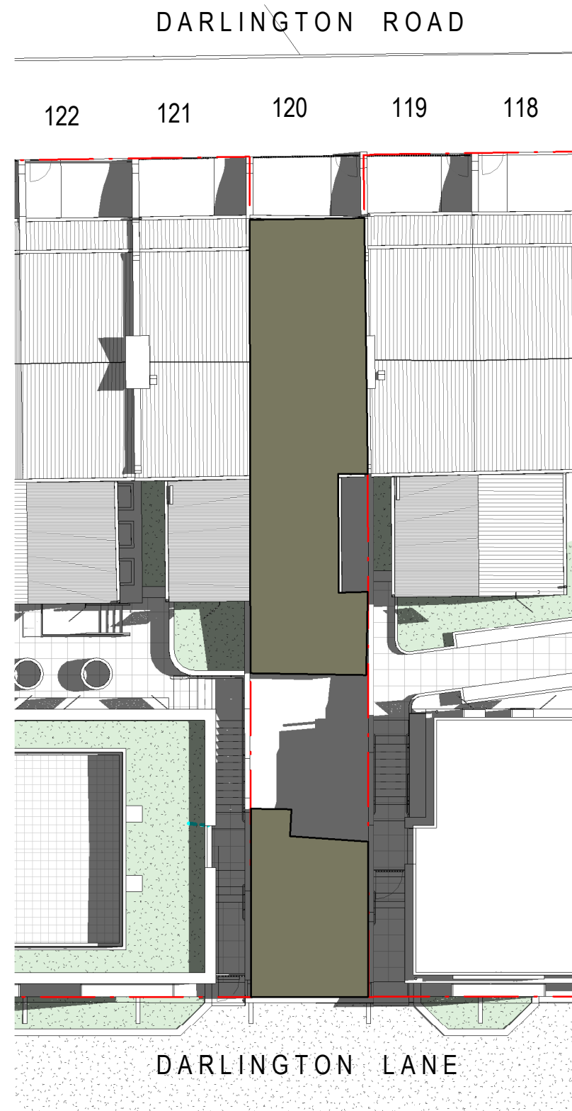
7 15 FEBRUARY 10AM 1:200 BETWEEN 10AM - 3PM (INCLUSIVE) NO.120 DARLINGTON ROAD RECEIVES 5 HOURS OF SOLAR ACCESS TO AT LEAST 8SQM OF THEIR REAR PRIVATE OPEN SPACE. 3 HOURS ABOVE THE SYDNEY DCP REQUIREMENT OF MIN. 2 HOURS
