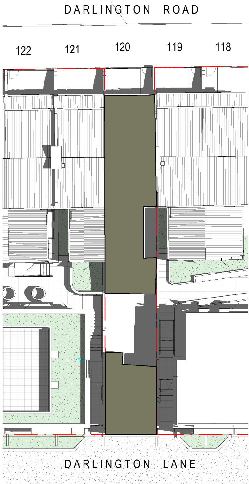
1 01 JANUARY 10AM 1:200 BETWEEN 10AM - 2.30PM (INCLUSIVE) NO.120 DARLINGTON ROAD RECEIVES 4.5 HOURS OF SOLAR ACCESS TO AT LEAST 8SQM OF THEIR REAR PRIVATE OPEN SPACE. 2.5 HOURS ABOVE THE SYDNEY DCP REQUIREMENT OF MIN. 2 HOURS
