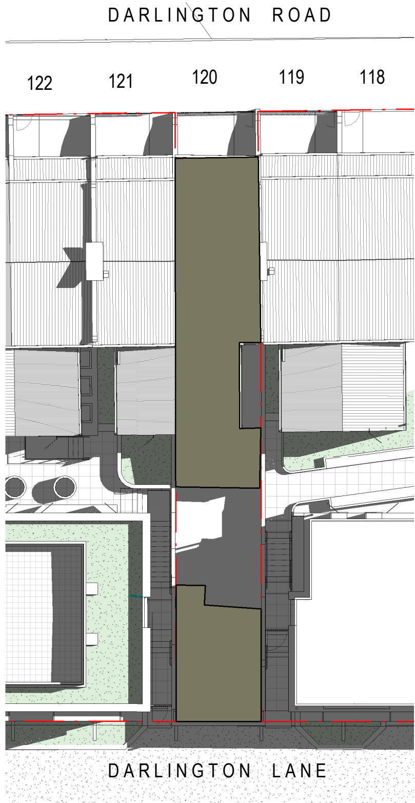
1 01 OCTOBER 9.30AM 1:200 BETWEEN 9.30AM - 2.30PM (INCLUSIVE) NO.120 DARLINGTON ROAD RECEIVES 5 HOURS OF SOLAR ACCESS TO AT LEAST 8SQM OF THEIR REAR PRIVATE OPEN SPACE. 3 HOURS ABOVE THE SYDNEY DCP REQUIREMENT OF MIN. 2 HOURS
