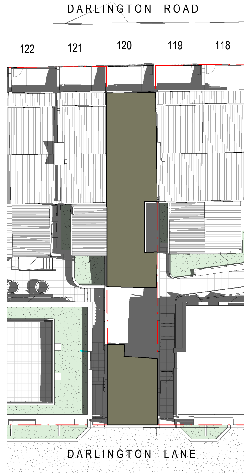
9 01 DECEMBER 9.30AM 1:200 BETWEEN 9.30AM - 2.30PM (INCLUSIVE) NO.120 DARLINGTON ROAD RECEIVES 5 HOURS OF SOLAR ACCESS TO AT LEAST 8SQM OF THEIR REAR PRIVATE OPEN SPACE. 3 HOURS ABOVE THE SYDNEY DCP REQUIREMENT OF MIN. 2 HOURS
