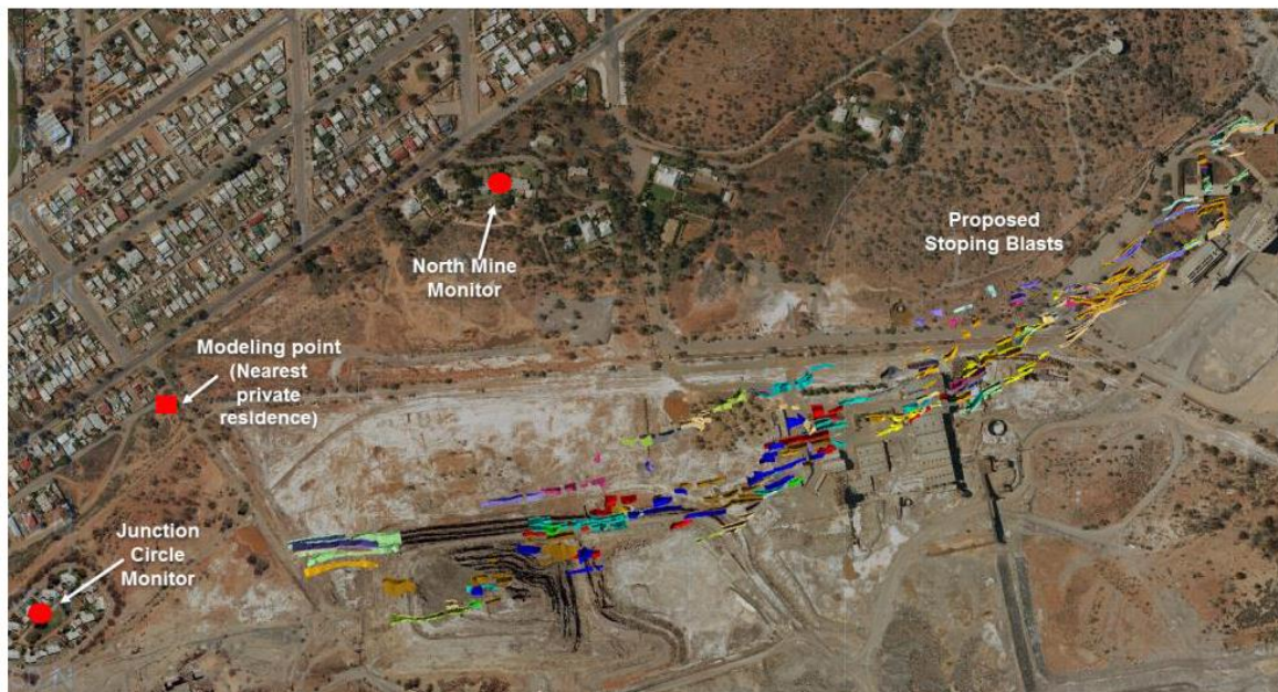
Figure 3.4: Plan showing stope locations with respect to monitors and private residences.
