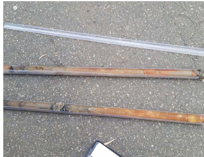
Material recovered from BH49, bitumen and roadbase with organic matter underlain by natural red/light brown mottled clay.
