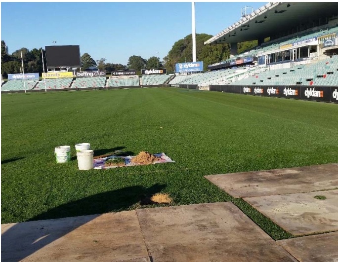
Sampling on the field facing south. Surface grass was cut and removed prior to drilling. Plywood used for track rig
