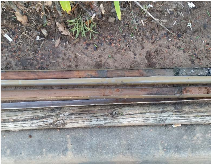
Push tube from BH01. Material recovered was bitumen and roadbase underlain by red/brown natural clay.
