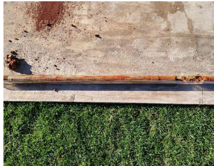
Natural material encountered at every location on the field consisted of red/light brown to white mottled clay.
