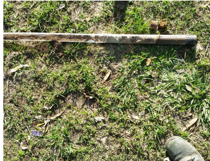
Material recovered from BH20, silty topsoil underlain by white silty sandy fill and natural red/brown clay
