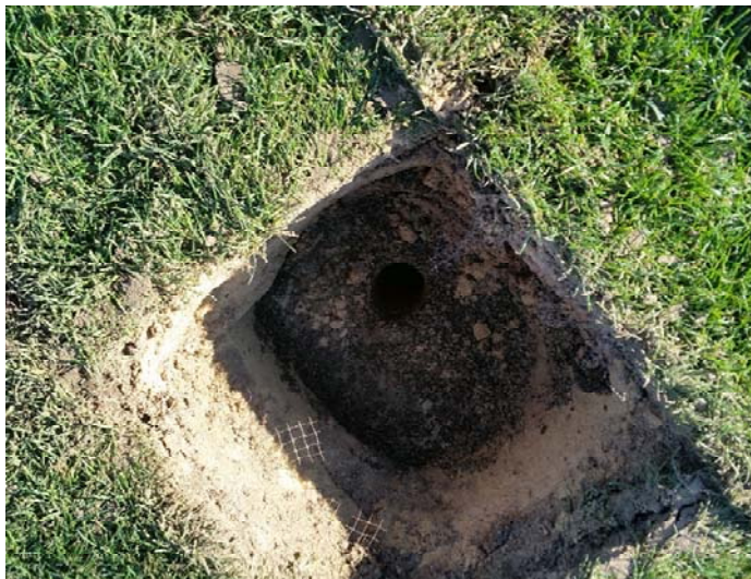
Fill material below grass at every location on the field, white sand underlain by gravel.
