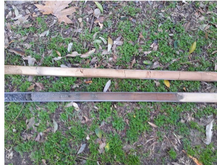
Material recovered from BH10. Bitumen and roadbase underlain by reworked clay and sand.
