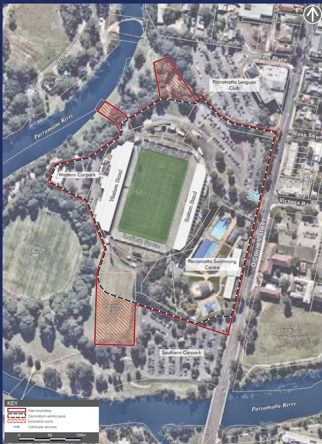
Demolition works area with exclusion zones
