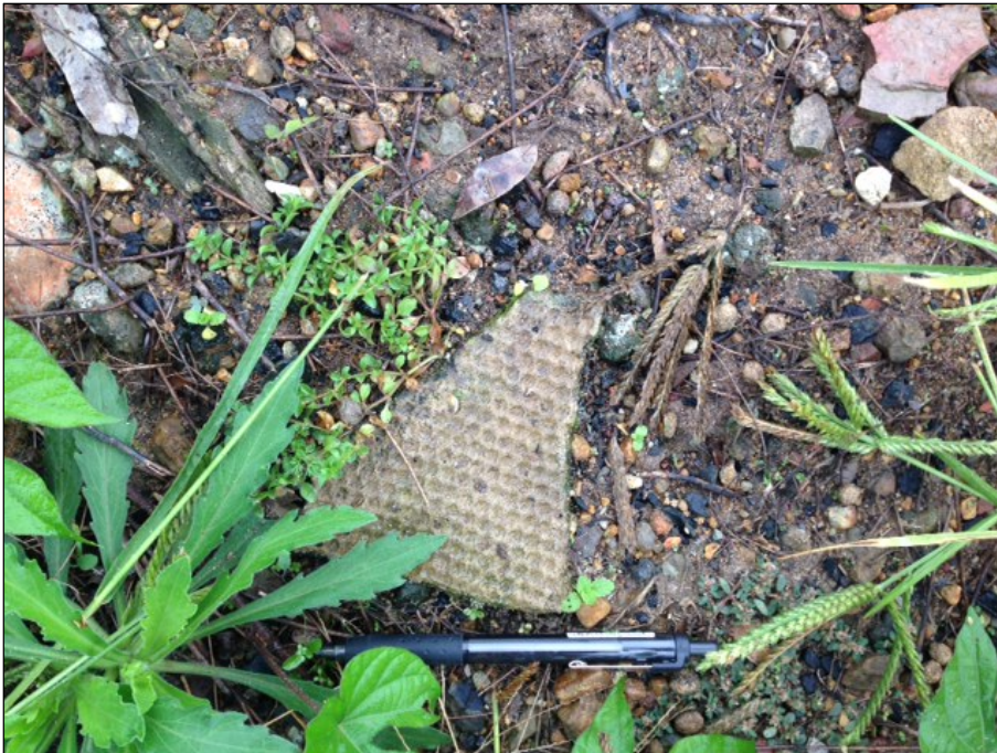
Figure 12: Fibro fragment observed adjacent to the southern site boundary (sample location A5)
