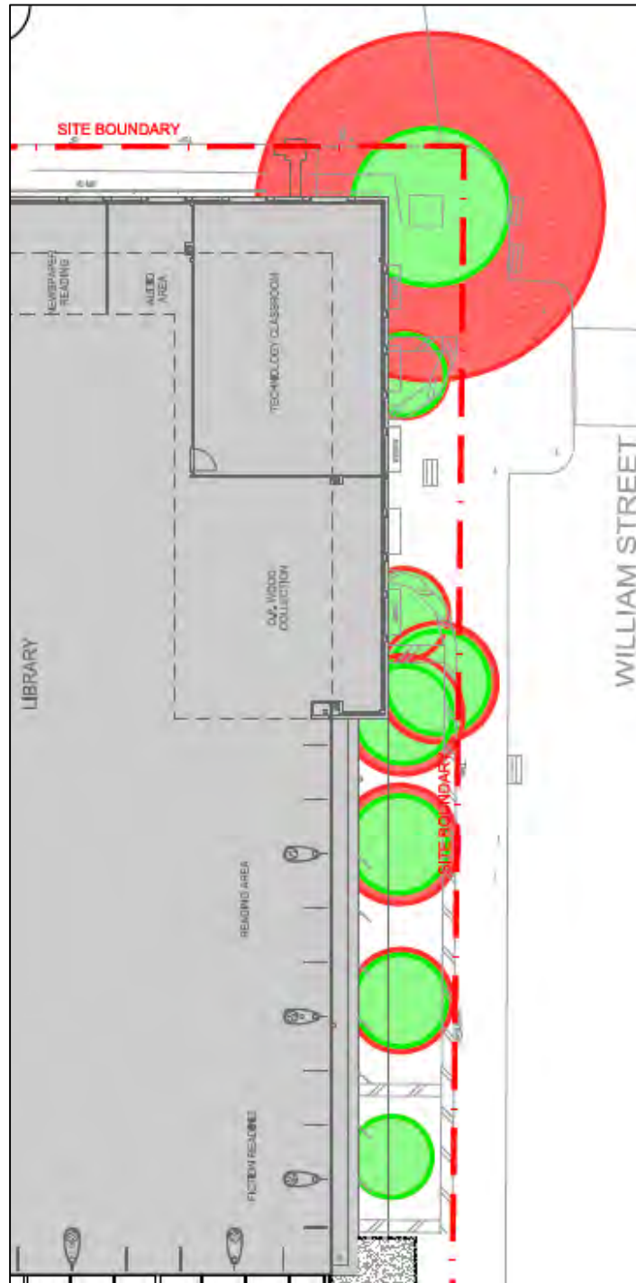
Fig. 26: Depicts tree numbers 33, 34, 35, 36, 37, 38, 39 & 40 which are able to be retained. Source: Diagram Tree Protection Zone Proposed. (Drawing Number A-SK-002), by Cox Architecture, Project 21304. 03.06.2016
