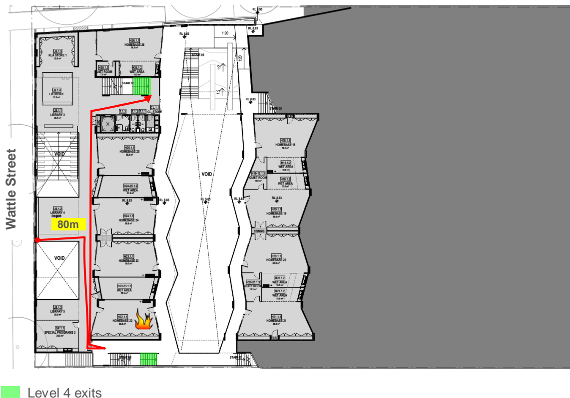
Figure 9 Fire scenario 1 – likely worst case travel distance by occupants in the event that an exit is blocked
