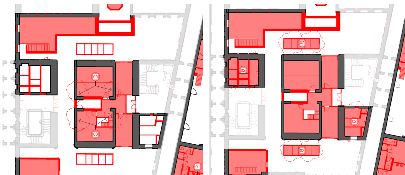
Figure 2 Approved Mod 9 Mezzanine Level demolition (left) and proposed Mod 15 Mezzanine level demolition (right) highlighting the WC changes
