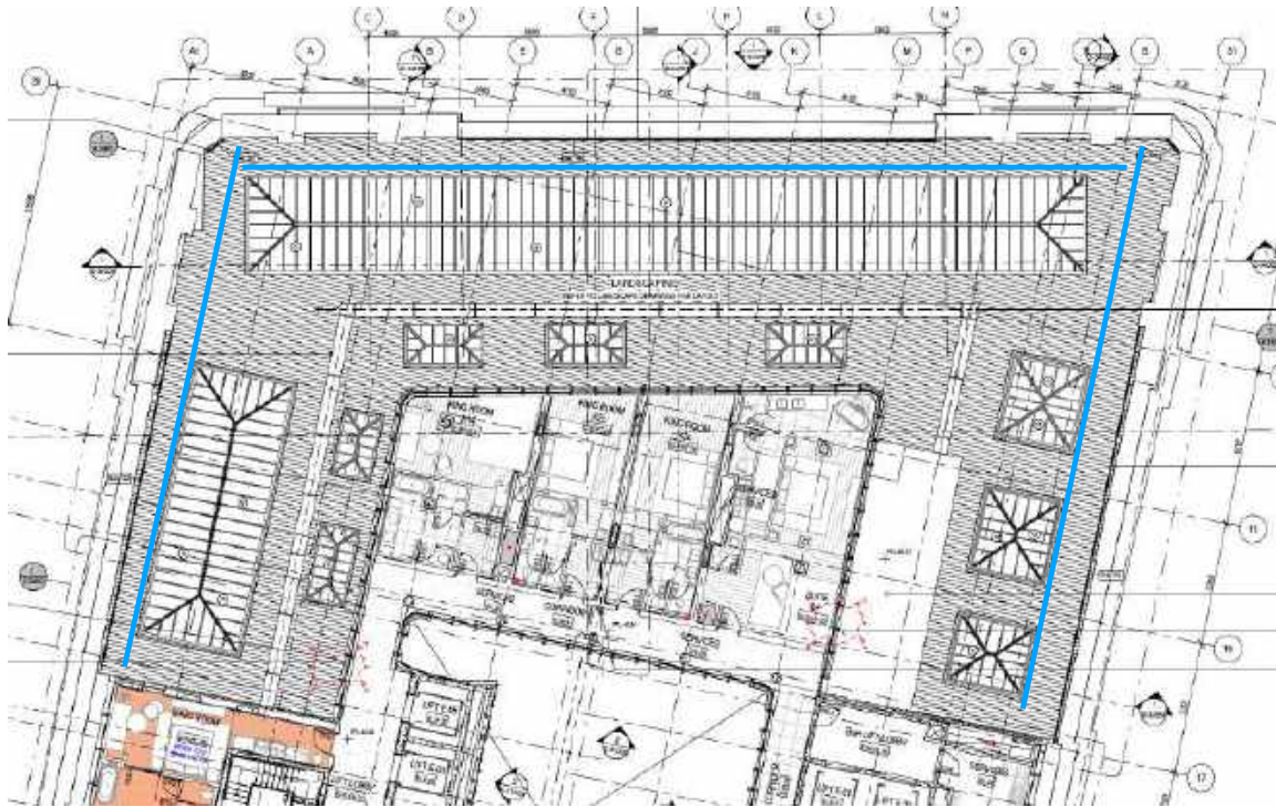
— Rope Access Rail on structural support beam
