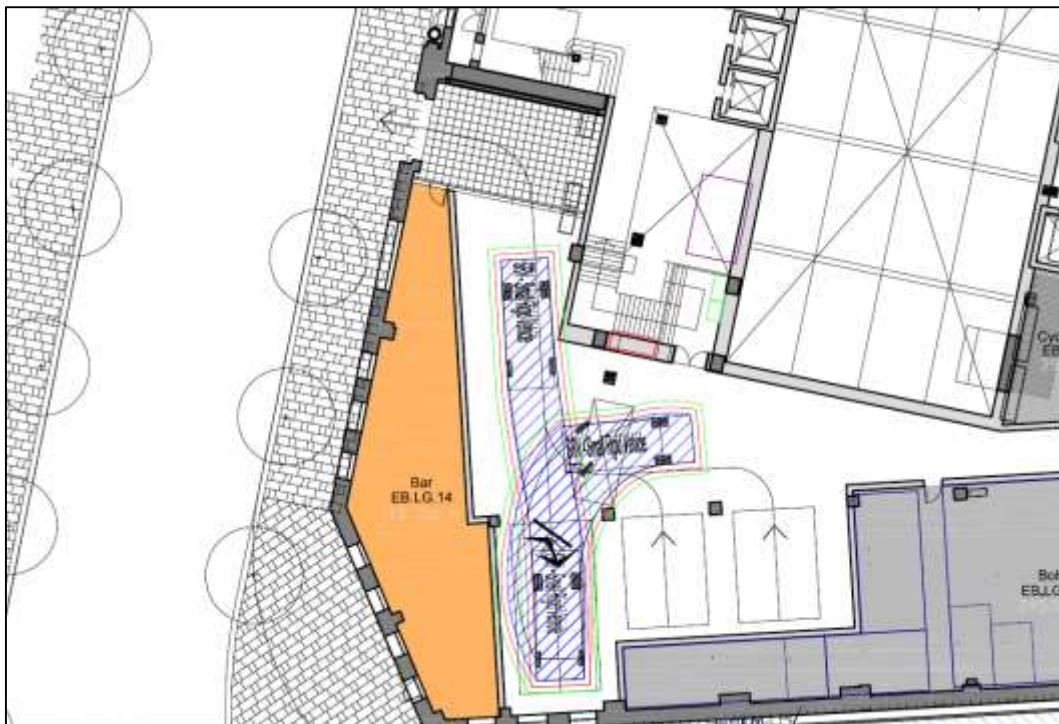
Figure 15 SRV manoeuvring in loading dock
