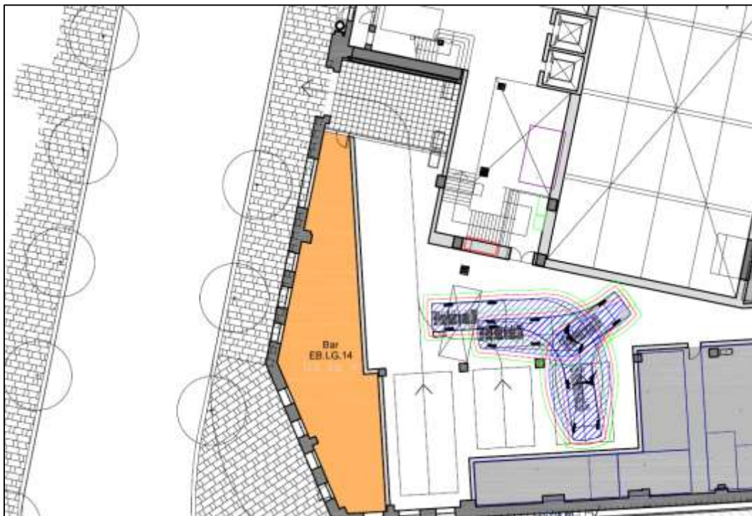
Figure 17 Van manoeuvring in loading dock
