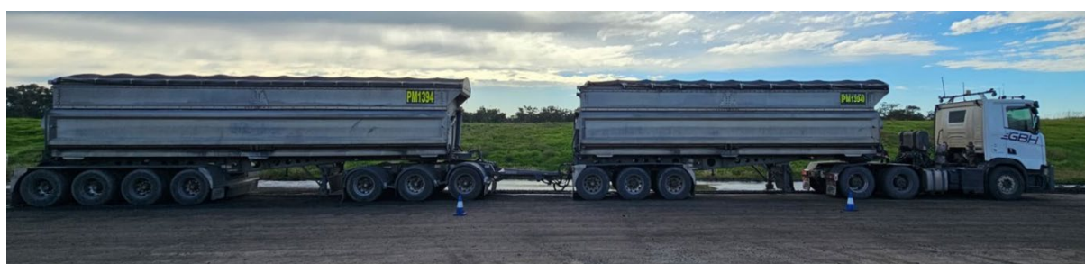
Figure 2.1: Typical Configuration of GBH A-Doubles
