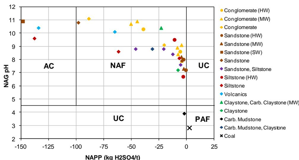
Figure 9: Geochemical classification plot for the different overburden and interburden material types (MW = Moderately Weathered, HW = Highly Weathered).
