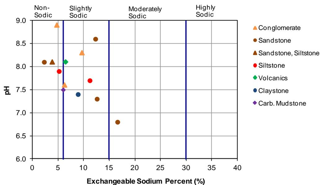
Figure 7: Sodicity ranking compared to pH for selected overburden and interburden drill-hole samples.
