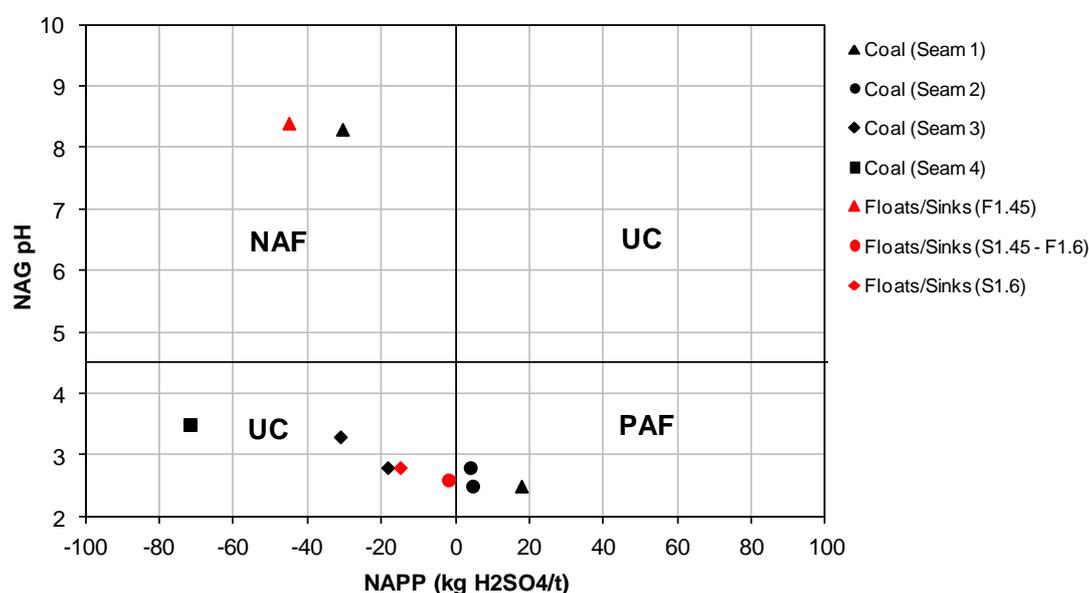
Figure 11: Geochemical classification plot for the coal seam and coal reject samples.
