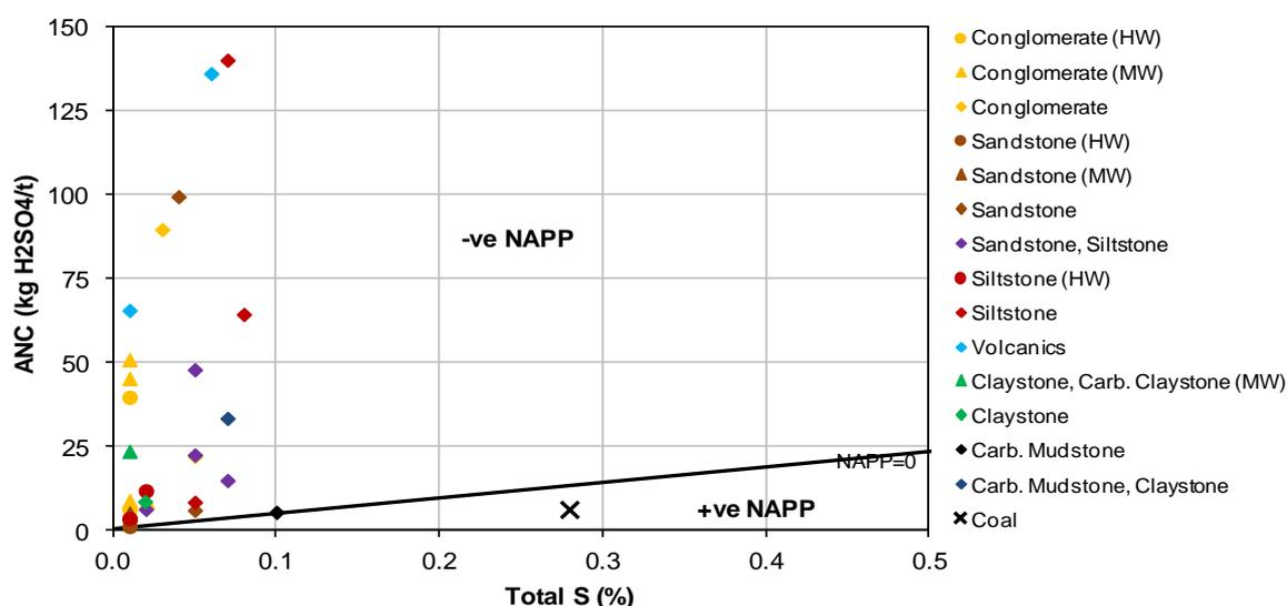
Figure 8: Acid-base account plot for the different overburden and interburden material types (MW = Moderately Weathered, HW =Highly Weathered).
