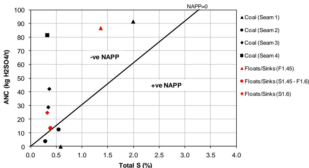
Figure 10: Acid-base account plot for the coal seam and coal reject samples.
