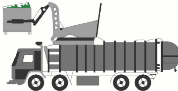
Front-lift-loading waste collection vehicle
