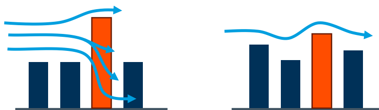
Figure 13: Schematic of flow pattern interference from surrounding buildings
