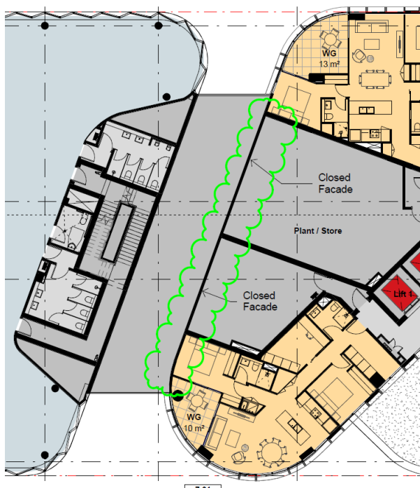
Figure 12 – Proposed screen to enclose plant on level 07
