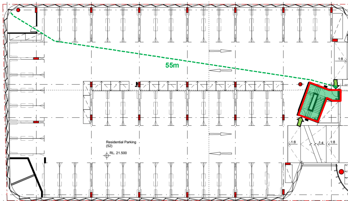
Figure 4 Maximum travel distance to nearest exit on the podium carpark levels 3 to 6
