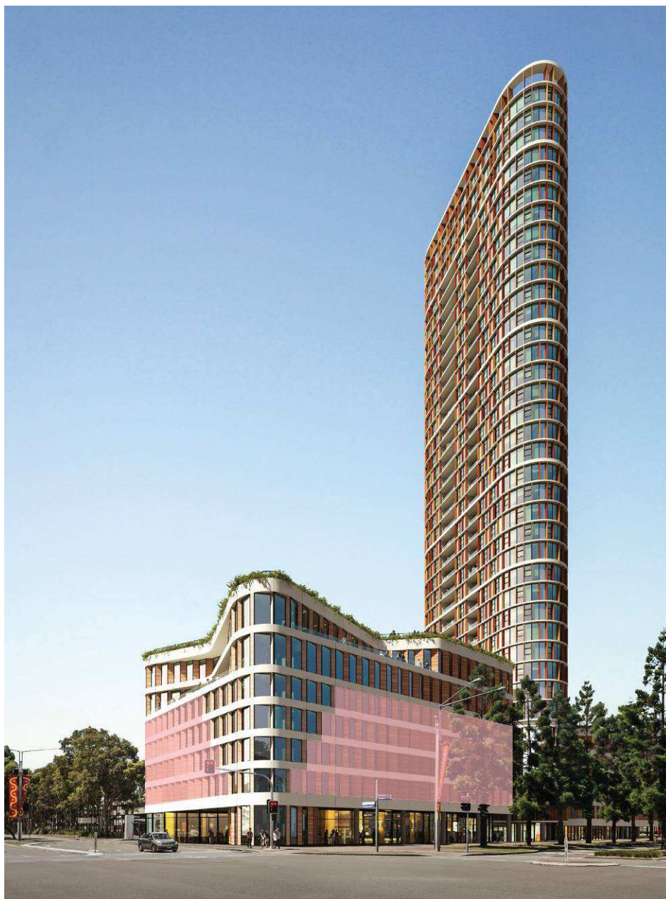
Figure 8 – Pink shading showing location of car park ventilation panels Source: Bates Smart
