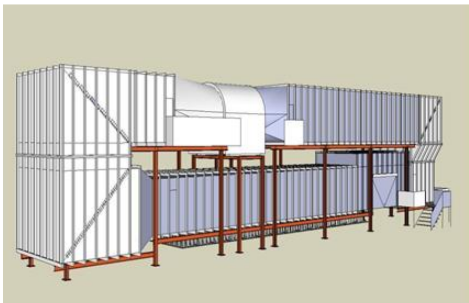
Figure 1: Schematic of the closed circuit wind tunnel
