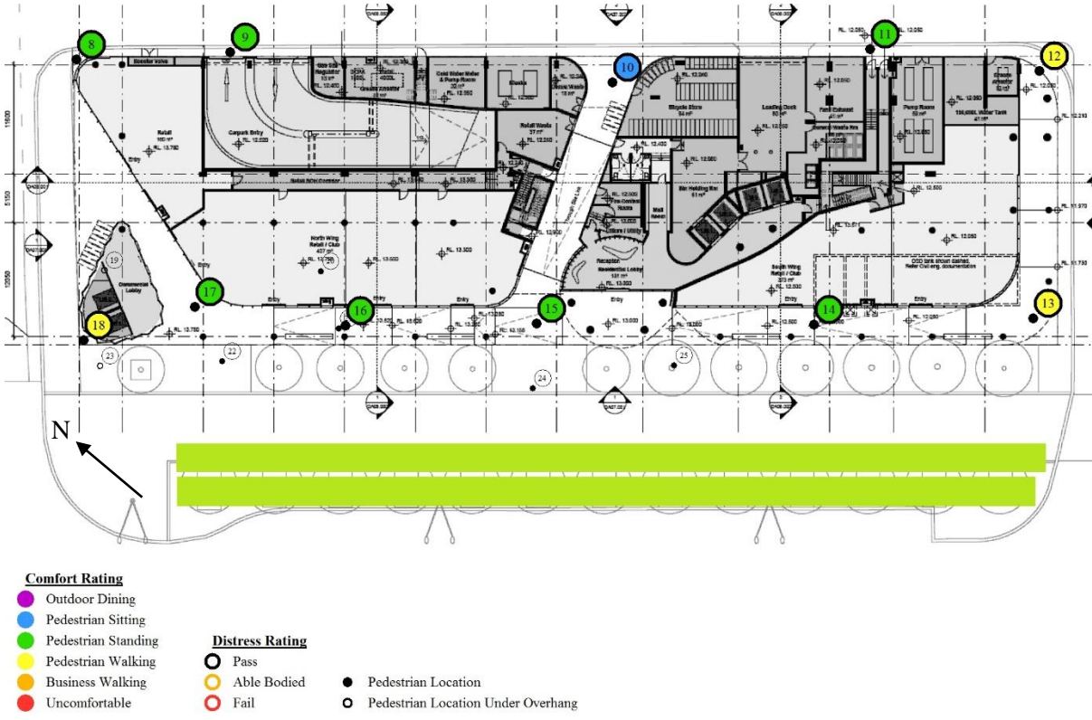
Figure 8: Pedestrian wind speed measurement locations with comfort/distress ratings – Ground floor of proposed configuration
