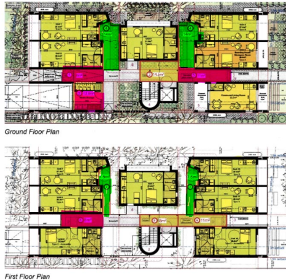
Figure 7: Floor Plans from Australex identifying relevant corridors / breezeways in red and green Source: Floor Area Plan, prepared by Hill Thalys dated September 2022
