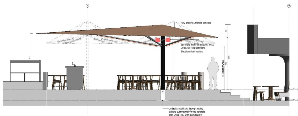
Figure 5: Indicative cross section showing existing umbrellas and proposed shade structure configuration
