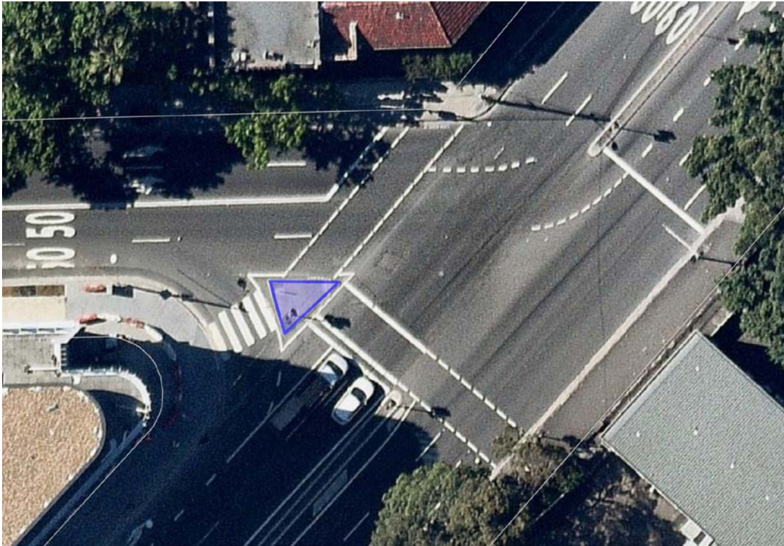
Figure 2.8: Pedestrian Island on City Road
