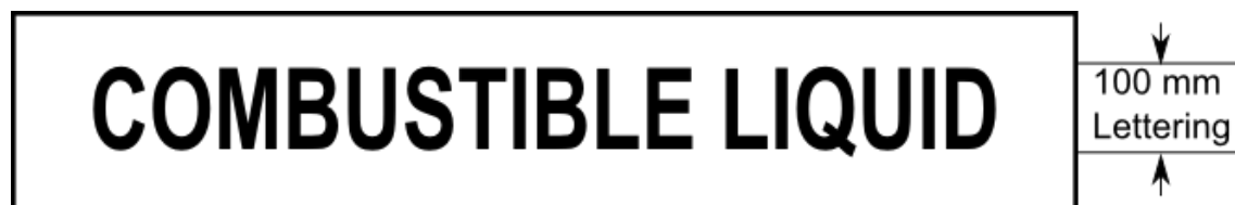
Figure 5-2: Combustible Liquid Placard
