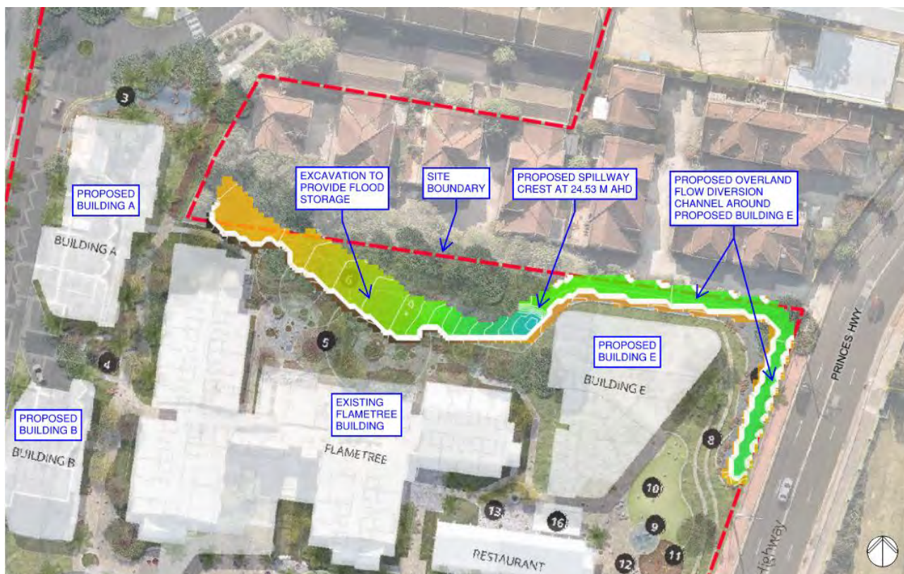
Figure 4-1 Proposed area of excavation and spillway at the stormwater line and overland flow diversion channel around Building E
