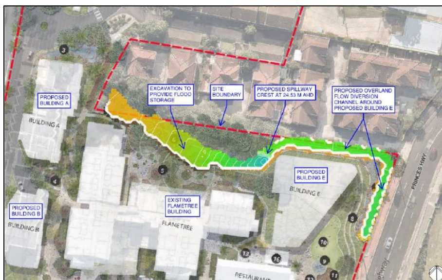
IMAGE 52 – PROPOSED AREA OF EXCAVATION AND SPILLWAY AT THE STORMWATER LINE AND OVERLAND FLOW DIVERSION CHANNEL AROUND BUILDING E (ACOR CONSULTANTS)
