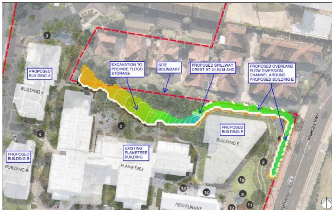
IMAGE 41 – PROPOSED AREA OF EXCAVATION AND SPILLWAY AT THE STORMWATER LINE AND OVERLAND FLOW DIVERSION CHANNEL AROUND BUILDING E (ACOR CONSULTANTS)
