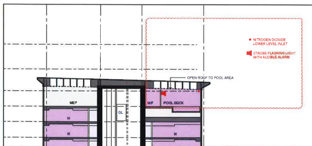
Figure 5 | Section showing proposed open roof area above the level 22 and 23 pool and bar area and location of NO 2 monitors and alarm (Source: Applicant's Architectural drawings).
