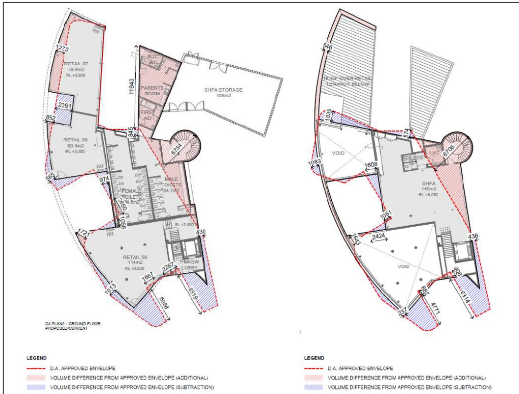
Figure 3 | Comparison of approved and proposed ground floor (left) and first floor (right) of the Property NSW building (Source: Applicant’s Modification report)
