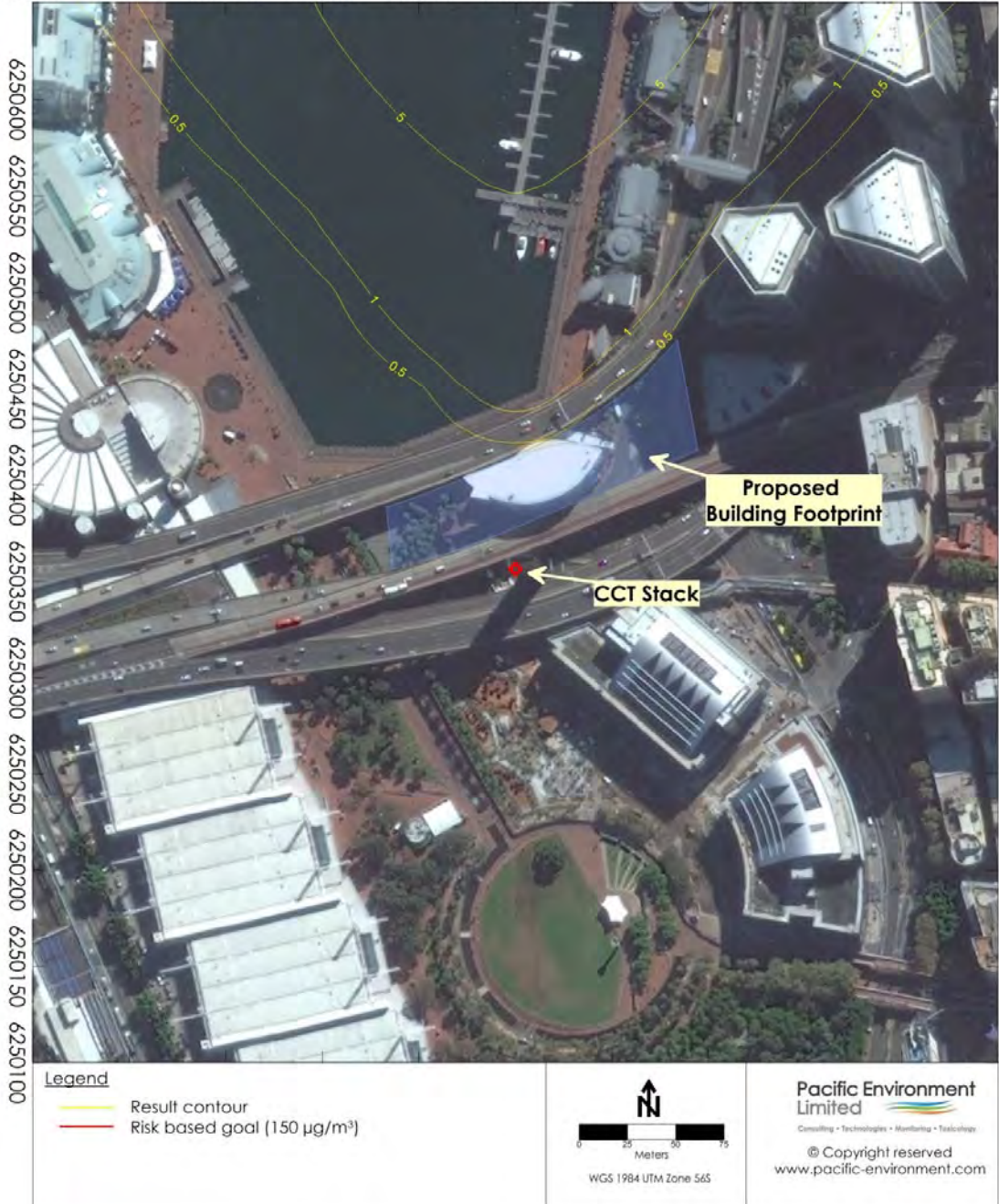
Ground Level – No Building Low Emissions Scenario – 1-Hour NO 2 Concentration (Goal – 150 µg/m 3 )
