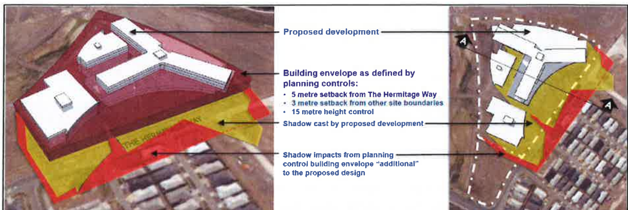
Figure 16: Overshadowing comparison of a compliant building footprint (overshadowing shown in red) and the proposed building footprint (shown in yellow) (Source: Applicant's EIS)
