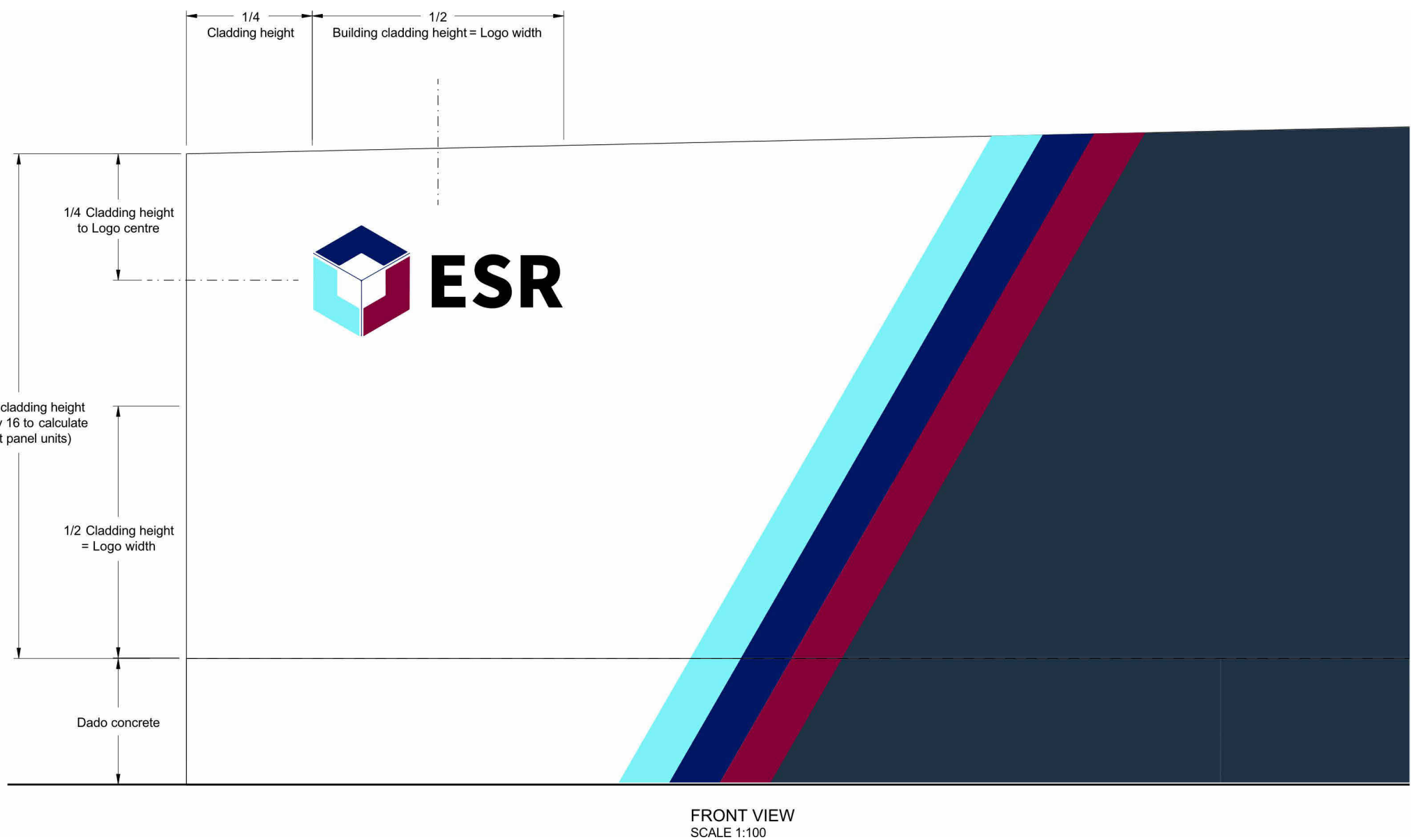
S3 SIGNAGE TYPE 3 CUSTOMER IDENTIFICATION FREESTANDING, ARTWORK AND COLOUR TO FUTURE DETAIL. NON ILLUMINATED
