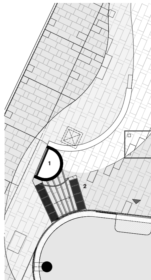
Plan of substation intake at Jones Street entry 1 - Intake ventilation stack, 2 - Stair to entry
