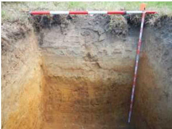
Plate 17. Soil profile in section, test pit 5, comprising historic fill overlying a coarse sand unit. Note the increasing clay content near the base indicative of Londonderry Clay in the vicinity of the base of excavations. .
