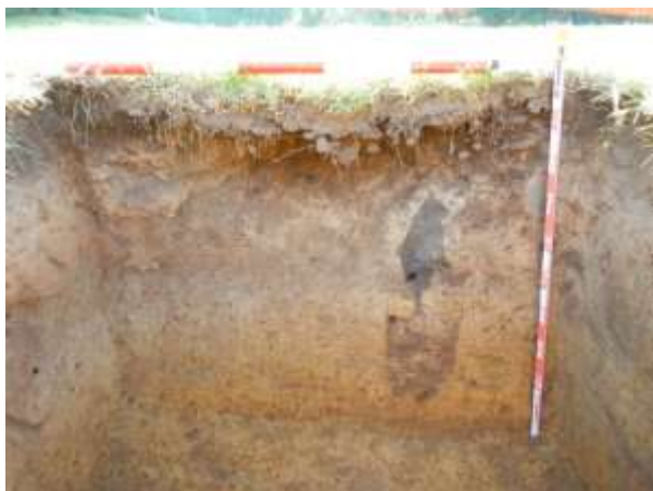
Plate 19. Soil profile in section, test pit 6, comprising historic fill overlying a coarse sand unit. Note the increasing clay content near the base indicative of Londonderry Clay in the vicinity of the base of excavations.
