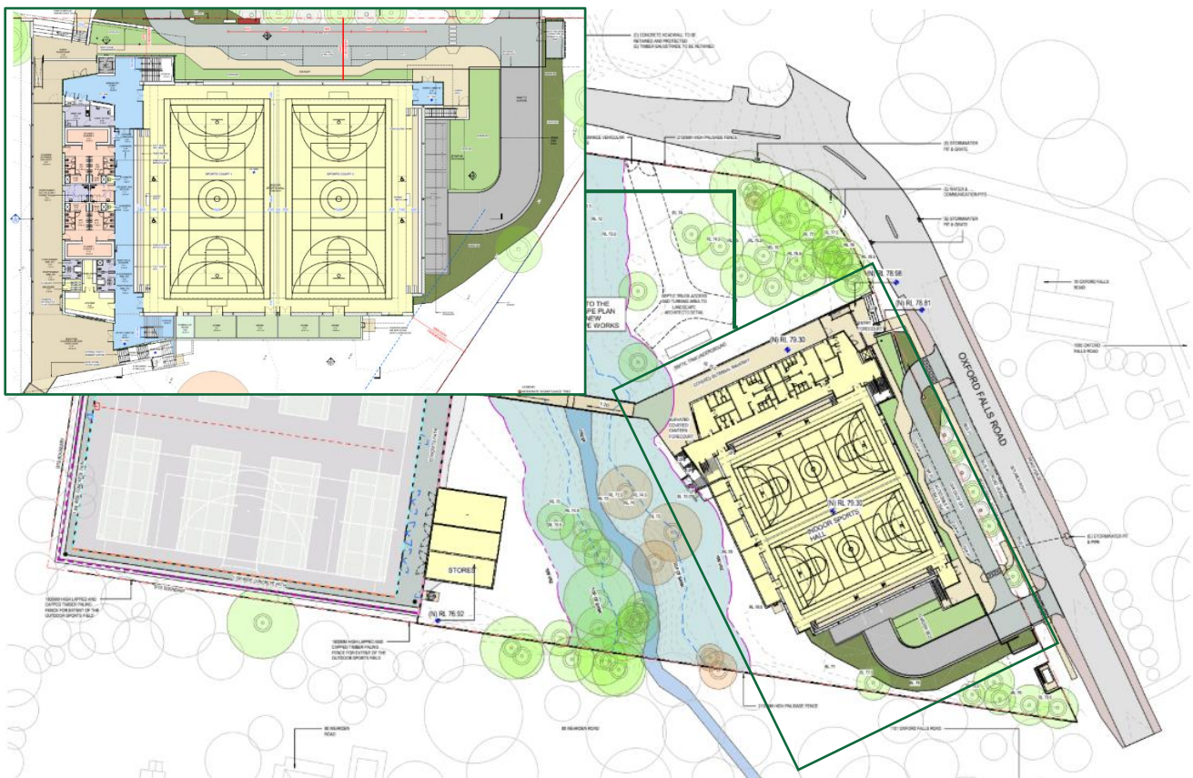
Figure 19 Site Plan with cut out to identify setback associated with indoor sports hall
