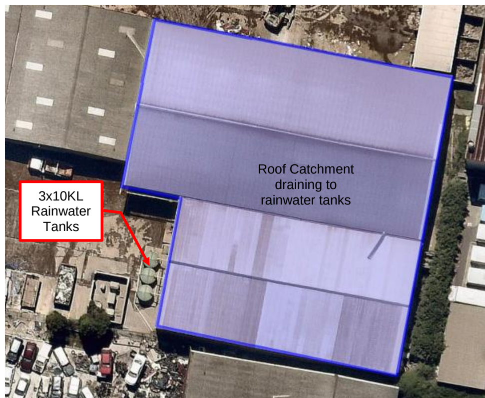
Figure 2-1 Rainwater Tank and Roof Catchment
