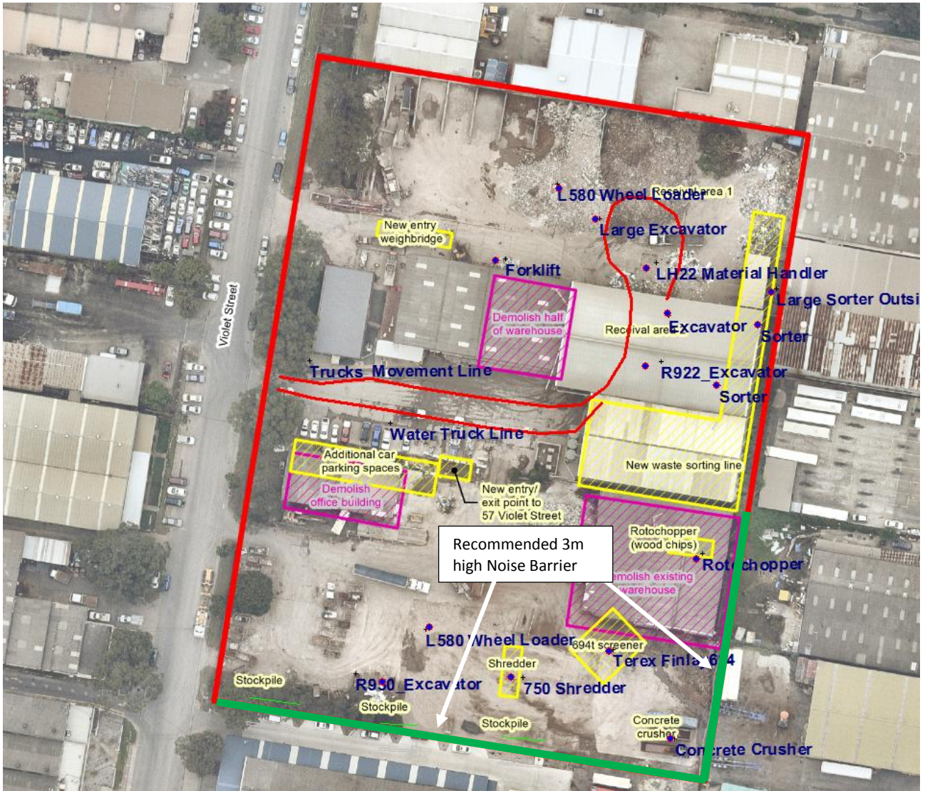
Figure 10: Location of Recommended 3 metre High Noise Barrier
