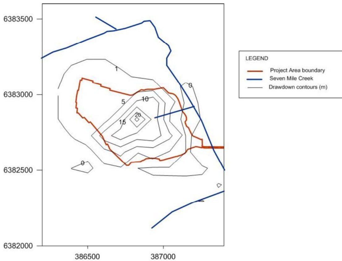
Figure 18 Drawdown in Layer 1 at the end of extraction period
