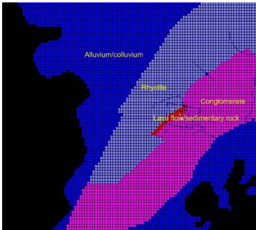
Figure 5 Map of hydraulic conductivity distribution in numerical model (Layer1)
