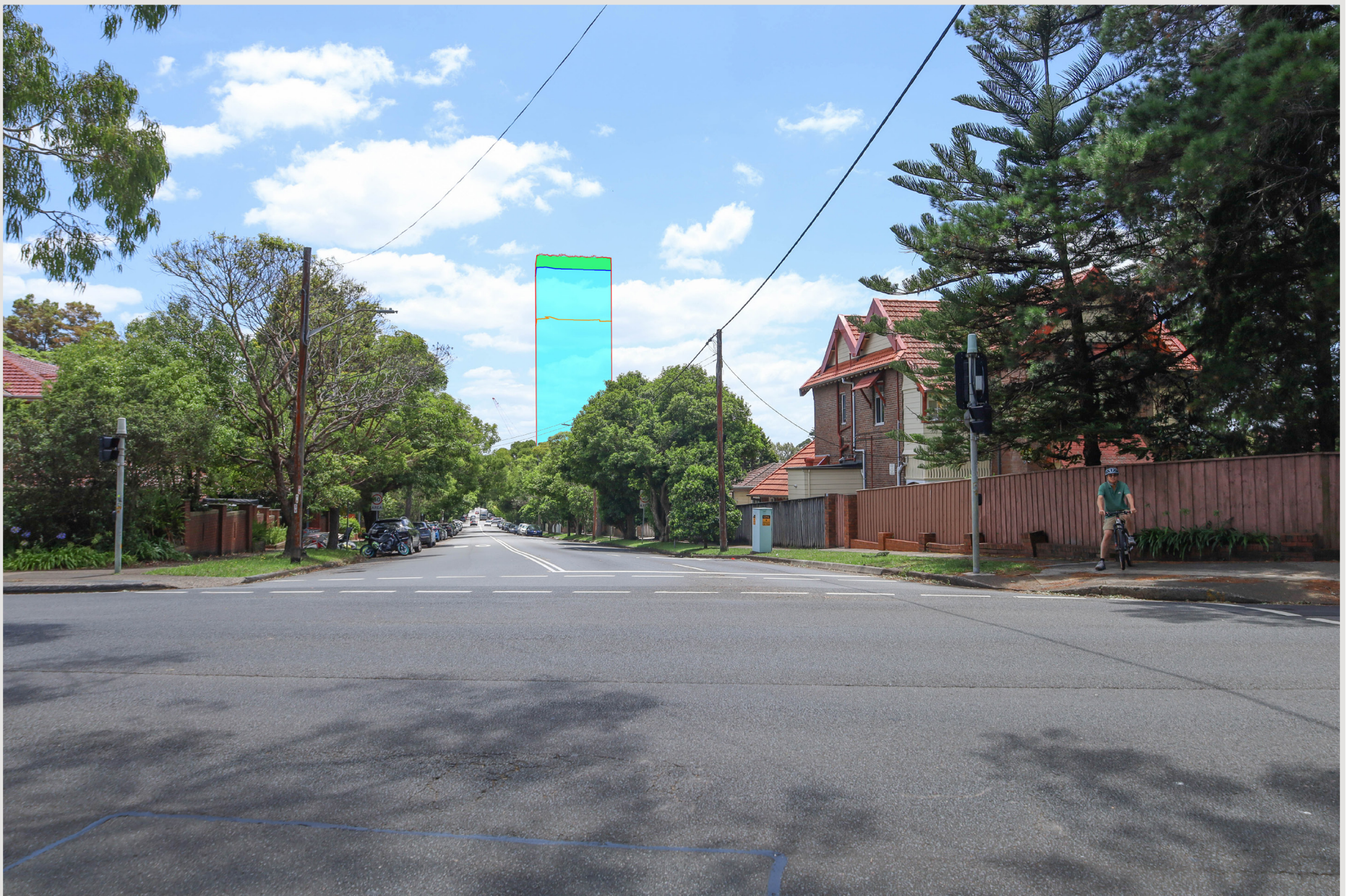
Visual Impact in cyan with red outline. WLEP 2012 + SEPP (Housing 2021) infill affordable bonus - max height: 88.4m - Blue line height indicator WLEP 2012 - max height: 68m - Orange line indicator
