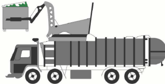
Front-lift-loading waste collection vehicle
