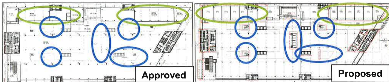
Figure 4: Upper Ground Floor level, showing proposed changes to the retail tenancies (in green) and changes to the stairs, lifts and atria (shown in blue) compared to the approved plans above (Source: FJMT)
