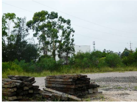
Plate 42. Deteriorated wooden sleepers for railway track placed in piles across the site. Facing east towards a large white industrial building present on the eastern boundary of the Intermodal site.
