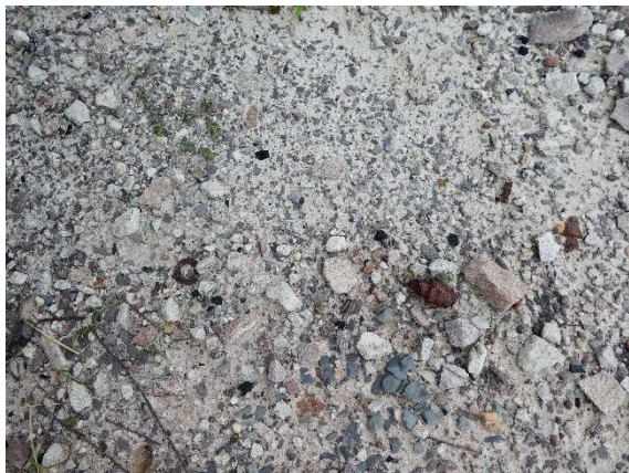
Plate 37. Ground fill material includes gravel, rock, dirt, and rusted metal work.
