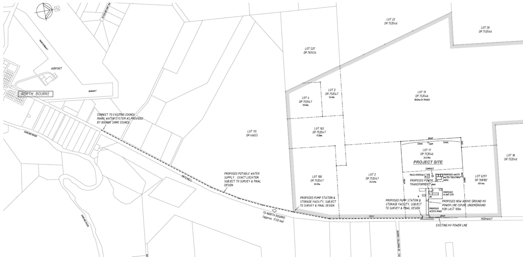
Figure 5: Reticulated water and electricity mains connections
