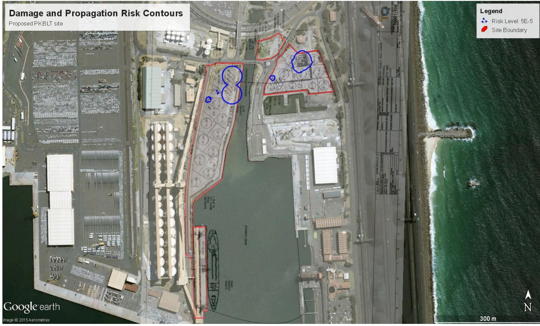
Figure 10.2: Damage and propagation risk contour – Stage 3
