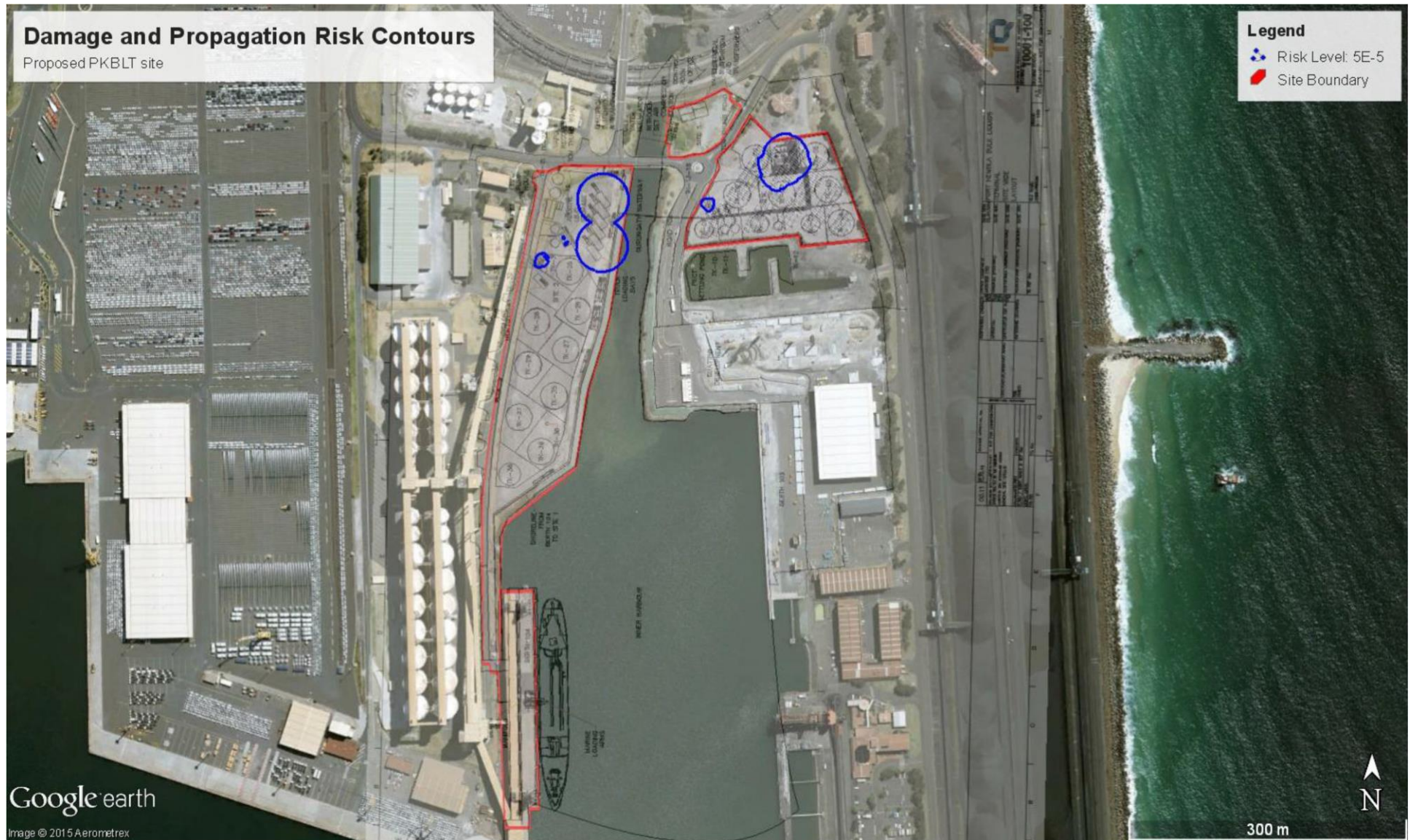
Figure 7-3 Damage and propagation risk contour – Stage 3 (Sherpa, 2015)
