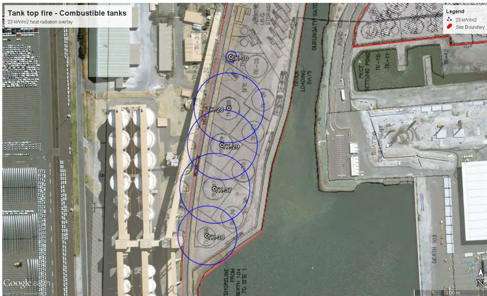
Figure 6: Combustible tank top fire – 23 kW/m 2 heat radiation
