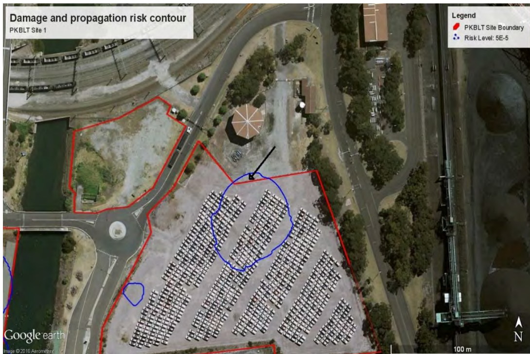
Figure 4: Damage and propagation risk contour (PHA extract)
