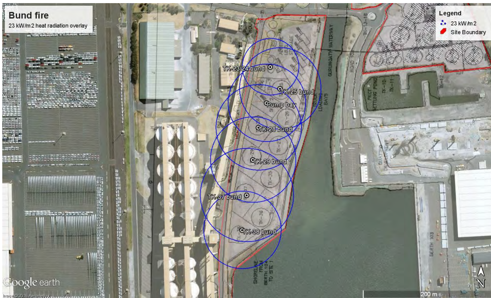
Figure 10: Bund fire – 23 kW/m 2 heat radiation
