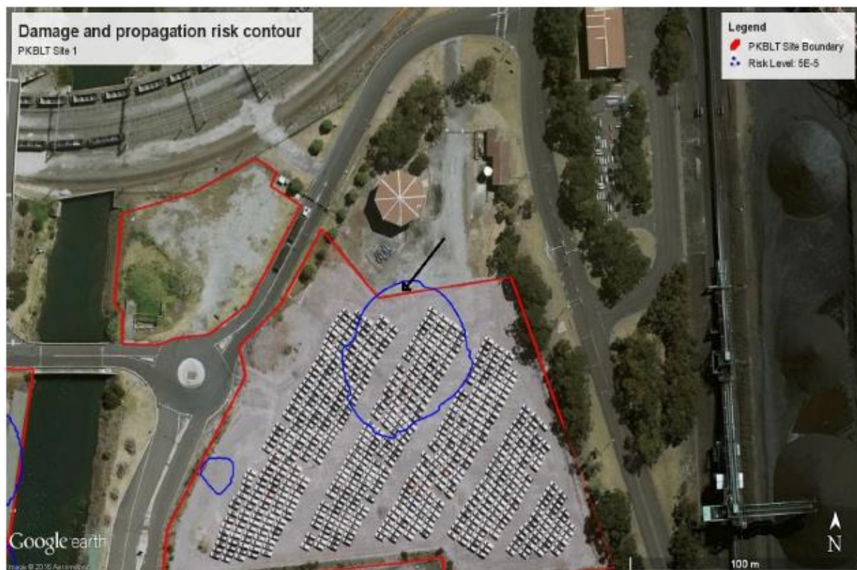
Figure 2 - Damage and propagation risk contour (PHA extract)
