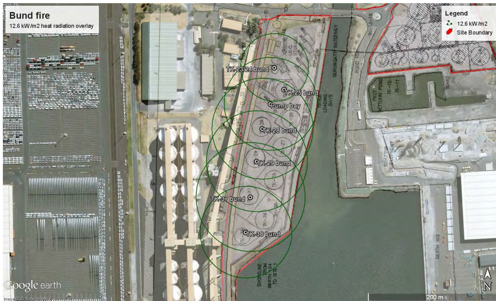
Figure 9: Bund fire – 12.6 kW/m 2 heat radiation
