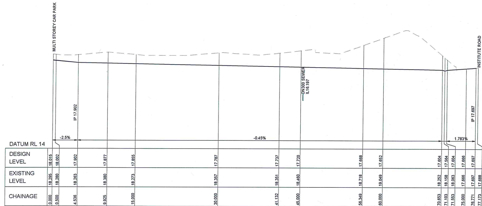
CARPARK EXIT ROAD (MC00) LONGITUDINAL SECTION HORIZONTAL SCALE 1:200 VERTICAL SCALE 1:50
