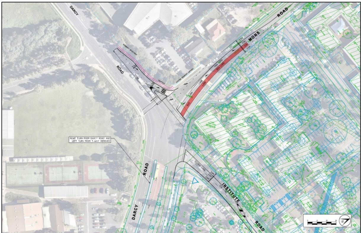
Figure 5: Proposed upgrade of Darcy Road/Mons Road/Institute Road intersection
